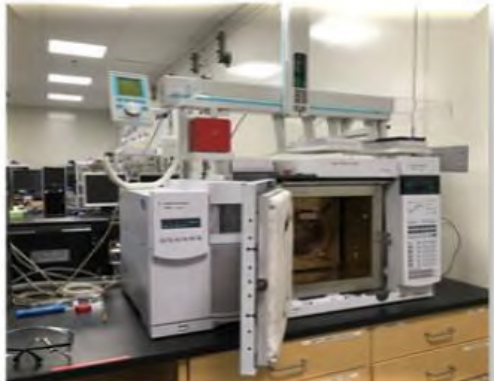
Figure 1. Head-space gas chromatography mass spectrometer at the BCIT Natural Health Products Lab used to measure ethanol levels (McIntyre, 2019).
