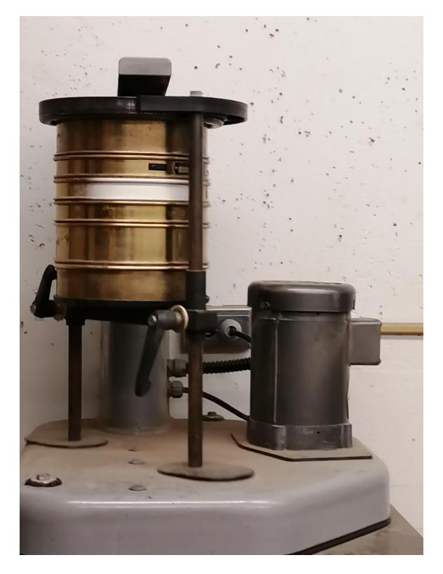
Figure 27. Photo of the sieve shaker sorting the grain sizes of a typical sample through sieve classes >2mm, (gravel), ) 0.5mm – 2mm (very coarse and coarse sand), 0.25mm – 0.5mm (medium sand), 0.125mm – 0.25mm (fine sand, 0.063mm – 0.125mm (very fine sand) and <0.063mm (silt and clay) for 5 minutes for a study for a study done on behalf of the Nature Trust of BC during a restoration project started in 2019 at the Nanaimo estuary, Nanaimo, BC
