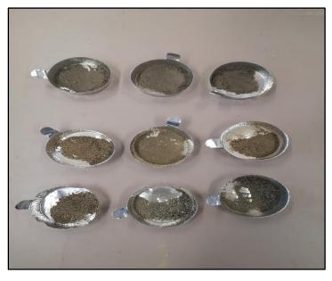
Figure 6. Sub-samples of a Soil Sediment Sample after testing for TOC vial LOI. Samples were taken from tidal channels during a restoration project began in 2019 by Nature Trust of BC in Nanaimo estuary, Nanaimo BC. Three samples were taken per site at each condition (before and after berm removal).
