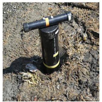
Figure 5. Photo of PVC corer used to extract sediment containing benthic invertebrate samples and soil samples for a study done on behalf of the Nature Trust of BC during a restoration project started in 2019 at the Nanaimo estuary, Nanaimo, BC.
