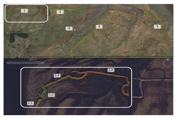
Figure 3. Maps showing parts of section one (white box) of the berm removal plan for year-one of the restoration project and the overall sections of the berm structures to be removed by the end of the restoration project in Nanaimo estuary, Nanaimo, BC. (Image: Adapted from deKoning, 2019)
