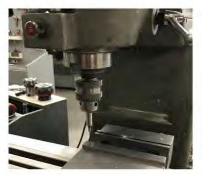
Figure 5.9. Milling Machine with Edgefinder
