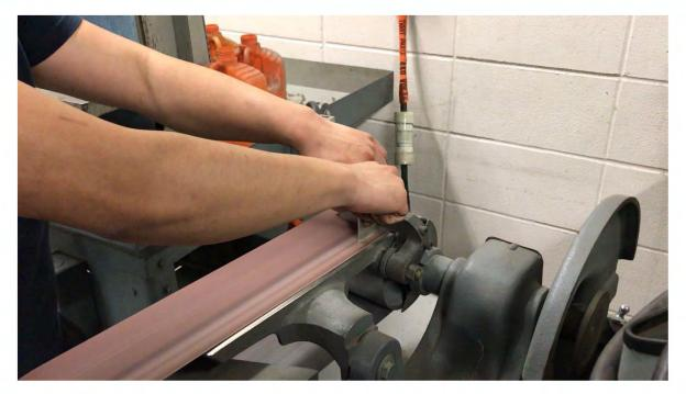
Figure 5.18. Removing Excess Material Using a Sanding Machine
