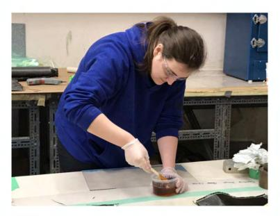
Figure 5.4. Mixing Epoxy Resin
