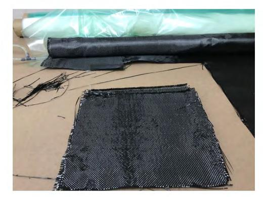
2. Squares of carbon fibre and Kevlar were cut from their storage rolls.
