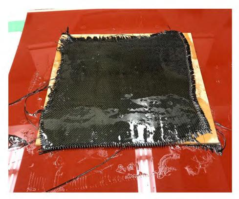
Figure 5.6. Sandwich Composite before the Epoxy Set
