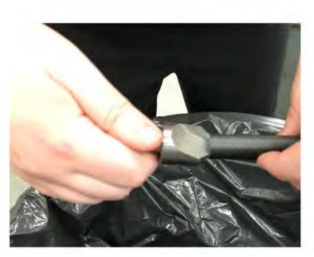
Figure 5.11. Deburring the Carbon Fibre Tubes
