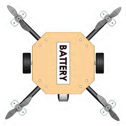
Figure 6.4. Top View of Final Drone SolidWorks Model
