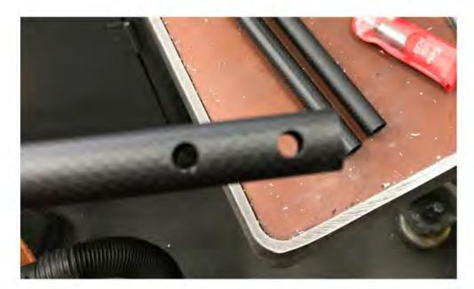
Figure 5.12. Completed Carbon Fibre Tube
