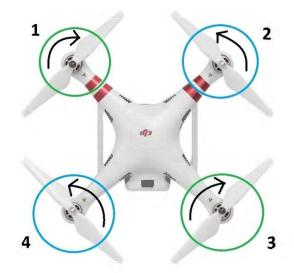
Figure 4.19: Basic Quadcopter Configuration [50]
