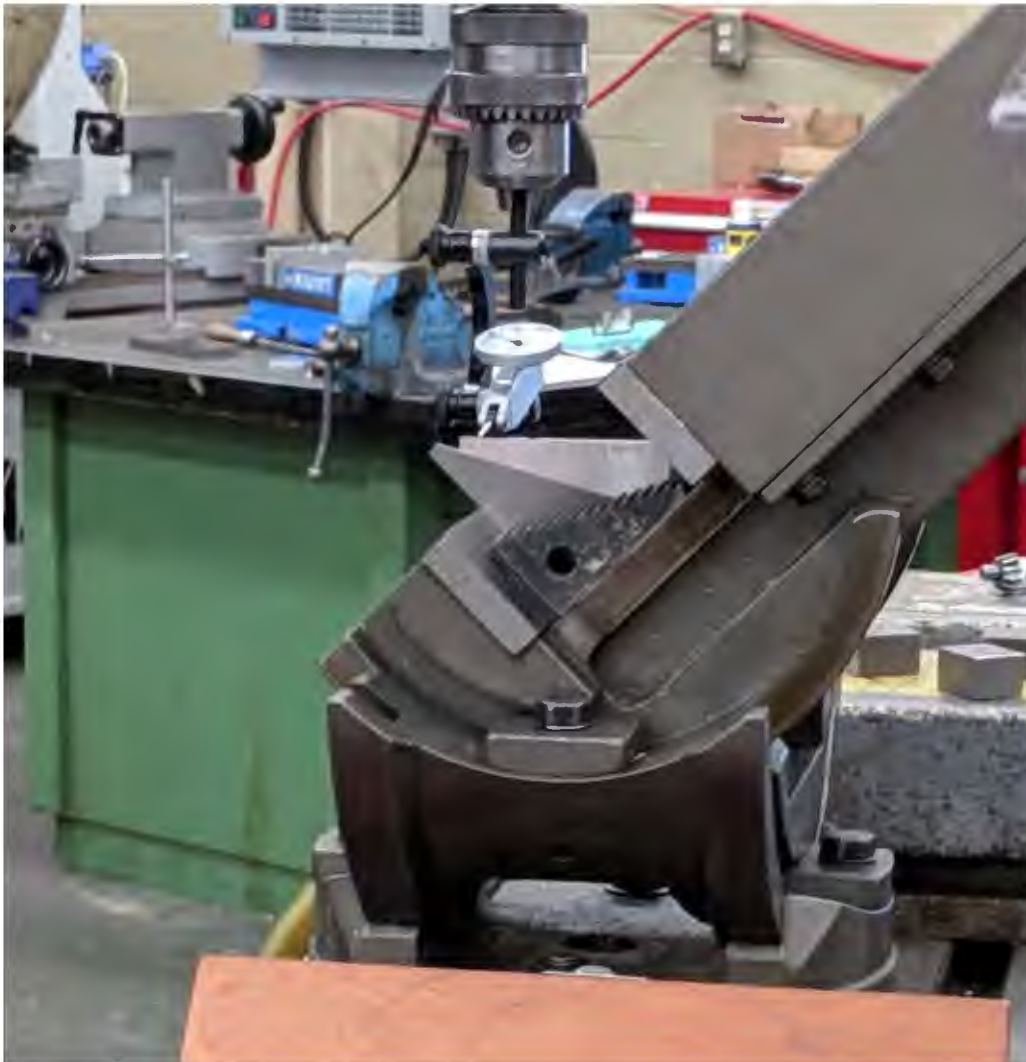
Figure 48 - Using a Dial Indicator for Calibrating 45° Vice
