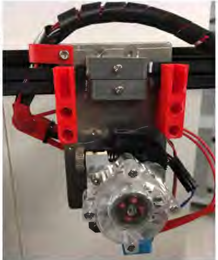
Figure 23 - Fully assembled printhead
