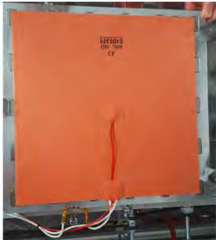
Figure 33 - 750W Silicone Bed Heater Glued to Underside of Print Bed
