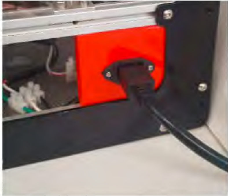
Figure 32 - IEC 320 Input Cable and Connector on Back Right-side of Printer
