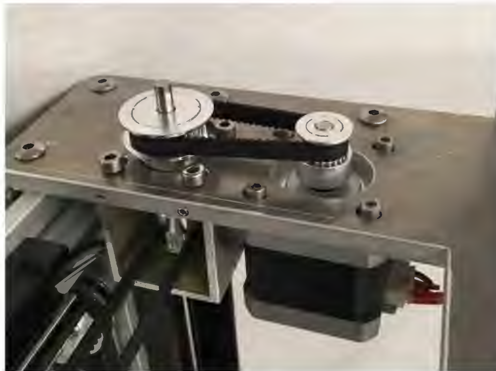
Figure 18 - Physical tensioning system view
