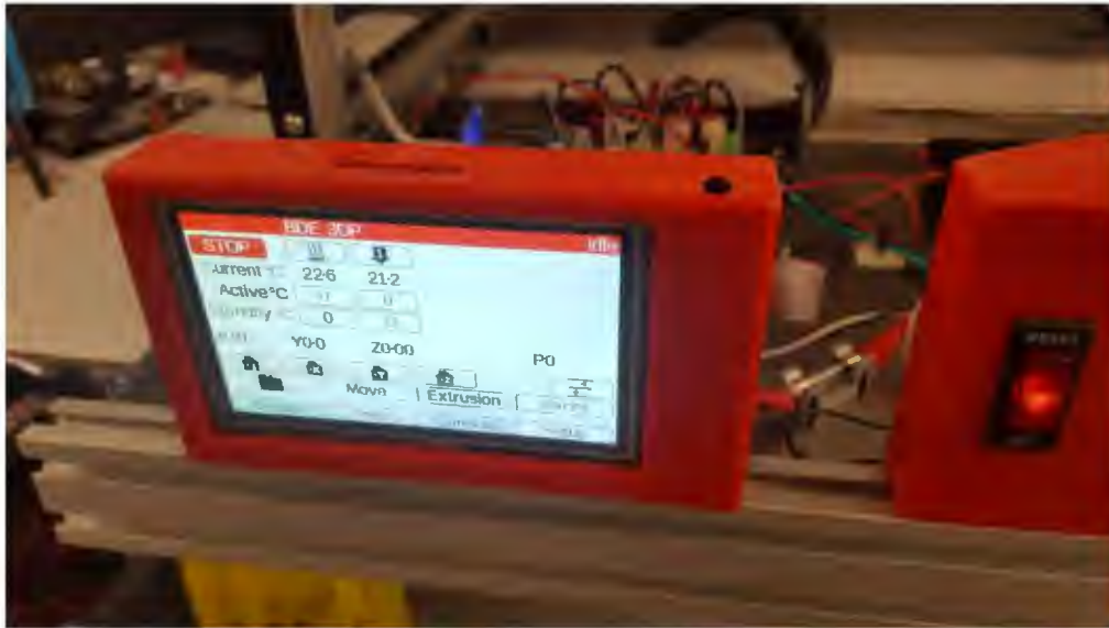
Figure 29 - Duet PanelDue 4.3" Touchscreen Monitor in 3D Printed Case
