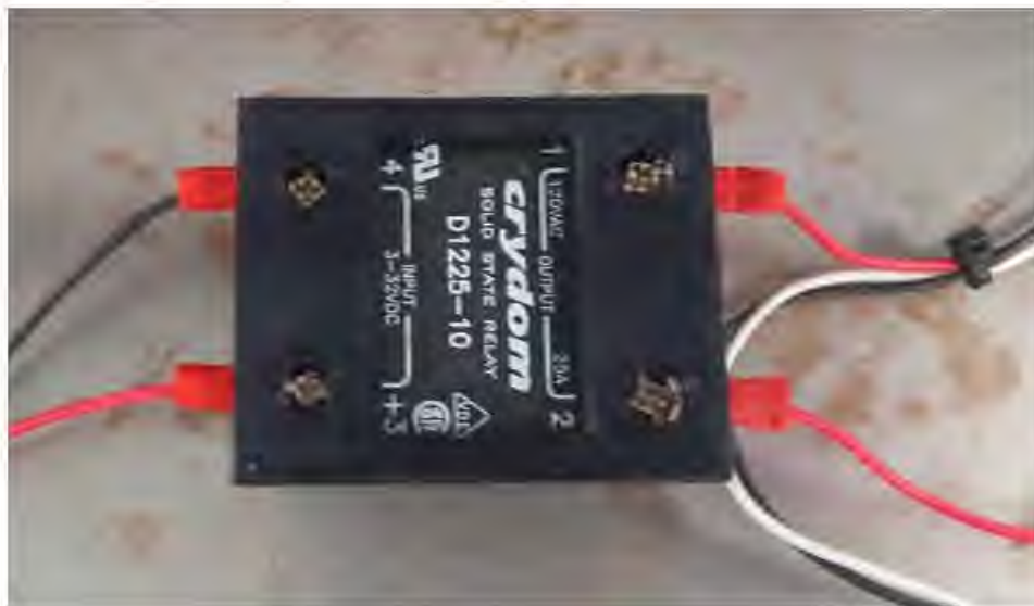
Figure 45 - 3D Printed Solid State Relay Cover (in black)
