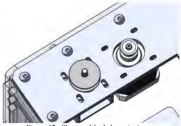
Figure 17 - Slots used for belt tensioning
