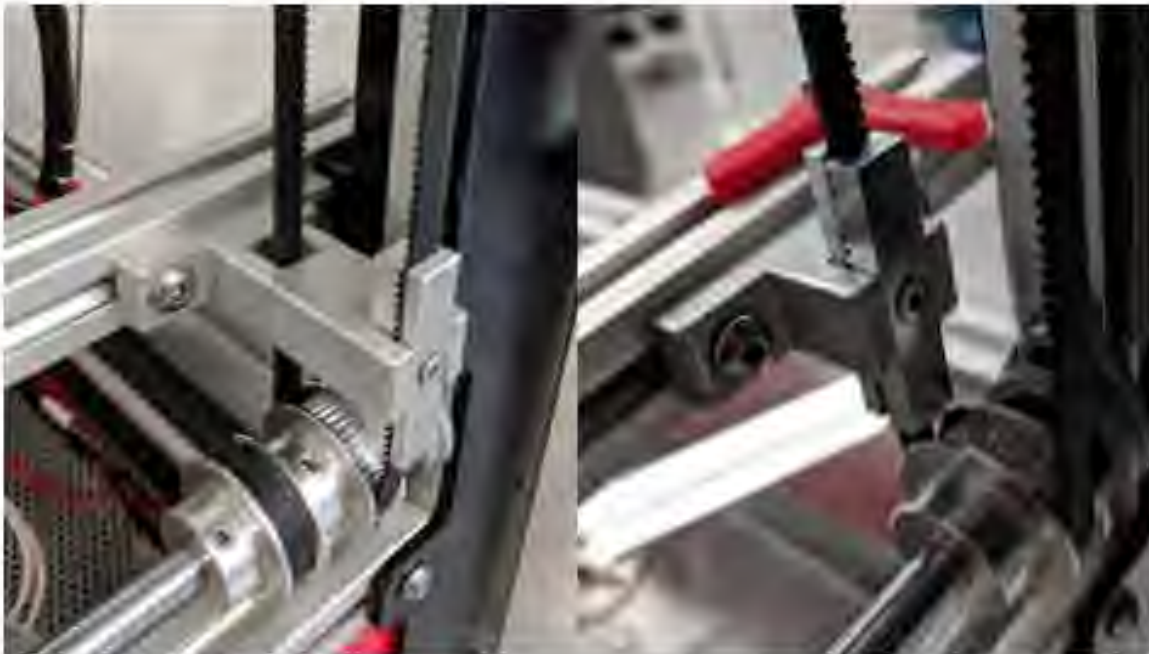
Figure 7 - Vertical Span Belt Clamps
