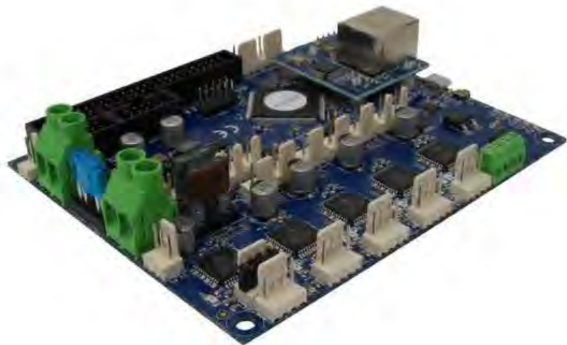
Figure 28 - Duet 2 Ethernet Controller
