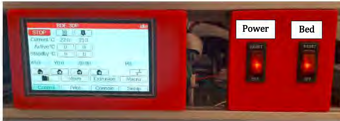
Figure 44 - Location of Switches and their Labels at Front of the Machine
