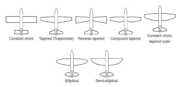
Fig 8: Picture showing the chord variation along wingspan [6]
