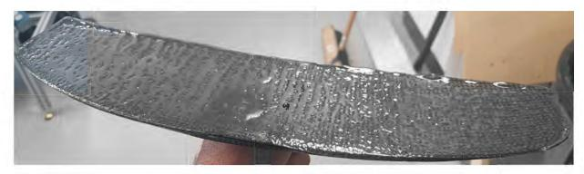
Figure 44: Non-uniform Epoxy Layer
