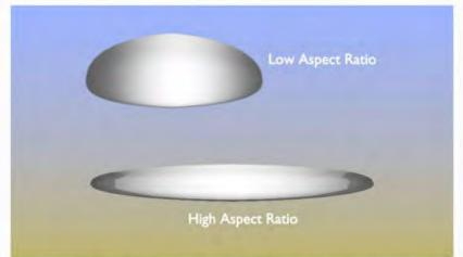
Aspect ratio is the ratio of the wingspan to the area of a wing. A wing with a short chord and long wingspan has a very high aspect ratio and vice versa.
