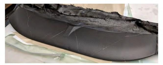
Figure 33: Wing after vacuum bagging
