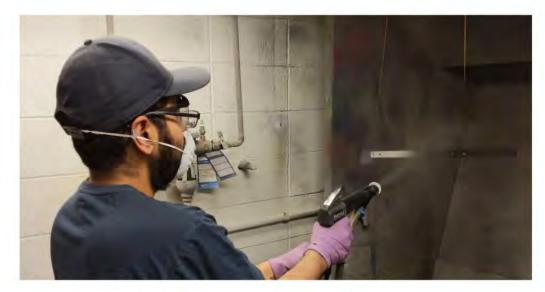
Figure 37: Powder coating process
