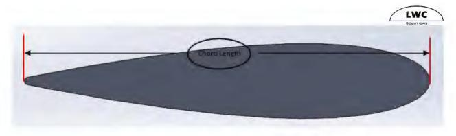
Fig 2: Cross section of a NACA 0018 wing profile, viewed from the side.
