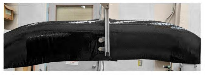
Figure 35: Exterior coating of epoxy added
