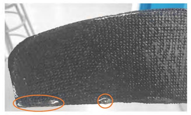
Figure 45: Epoxy Bubbles & Build-up
