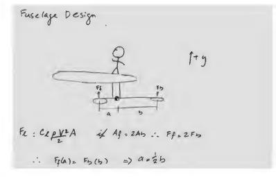
Figure 16: Diagram of the Centre of Mass of a Foil
