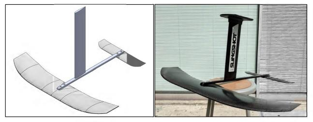
Figure 1: Final design compared to manufactured prototype
