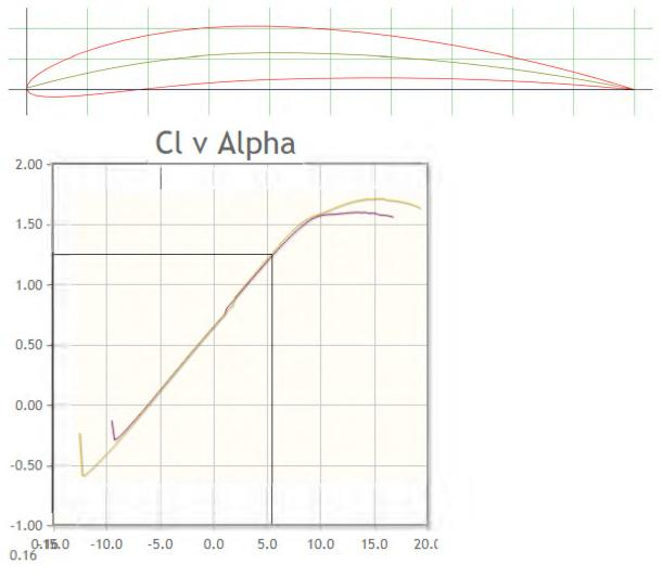
Figure 11: NACA 6409 9% Coefficient of Lift to Attack Angle [5]
