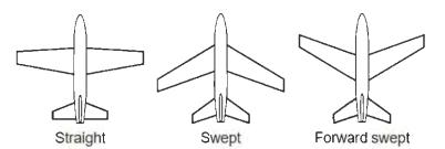
Fig 7: Wing sweep configuration examples [6]
