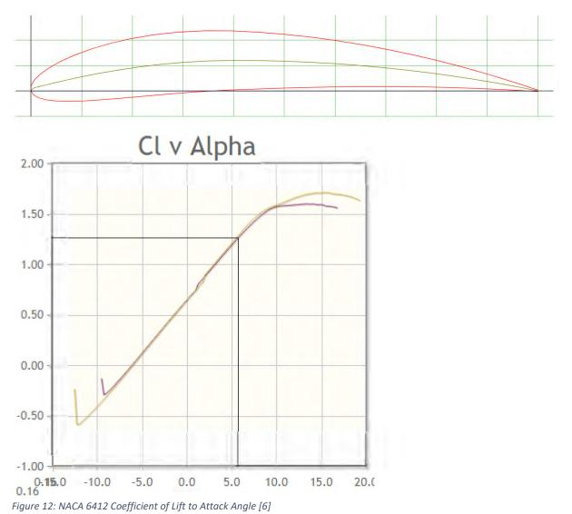
Because both profiles yielded very similar results, we decided to move forward with he NACA 6412 for the thickness of the wing. A thicker wing would make manufacturing easier down the line and more structurally sound.
