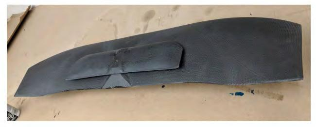
Figure 34: Hydrofoil after excess material removed
