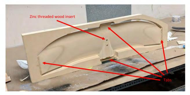
Figure 28: Finished CNC wing core
