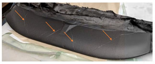
Figure 43: Folding on carbon-fiber layer
