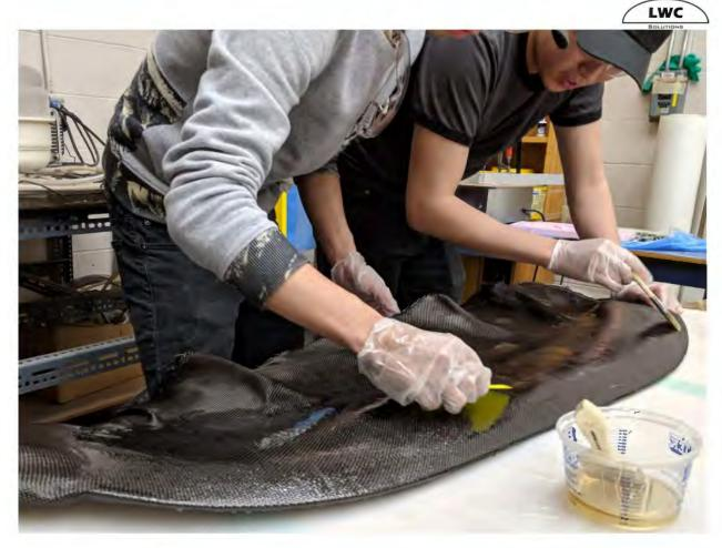
Figure 31: Carbon fiber layup process
