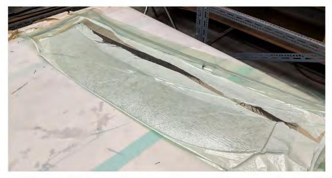
Figure 32: Vacuum bagging wing
