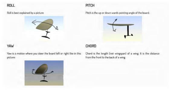
Figure 5: Three Rotational Freedoms of a Foil [2]
