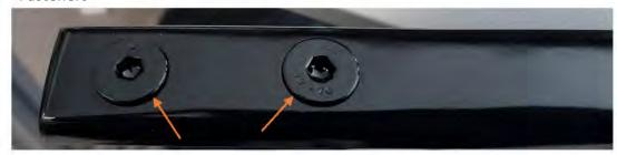
Figure 48: Powder Coated Fasteners
