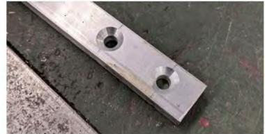
Figure 36: Drilled and countersunk connection holes
