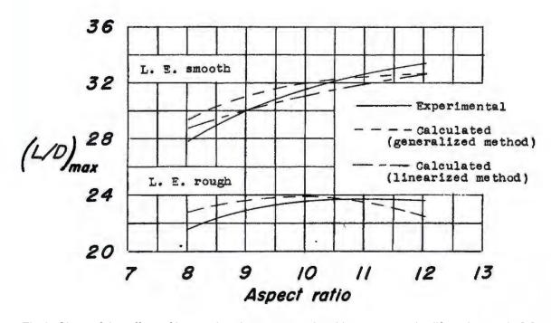
Fig 3: Chart of the effect of increasing the aspect ratio with respect to the lift to drag ratio [7] Increasing the Aspect Ratio of the front wing viewed from the side will result in a increase of the Maximum Operational weight because it produces more lift and allows for more weight.
