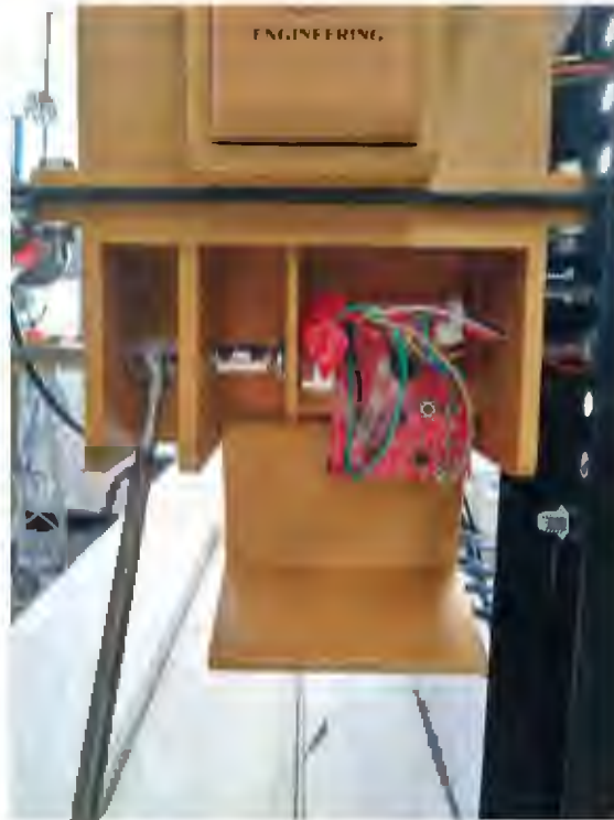
Figure 4-9: Potentiometer Coupled to Height Measurement Paddle
