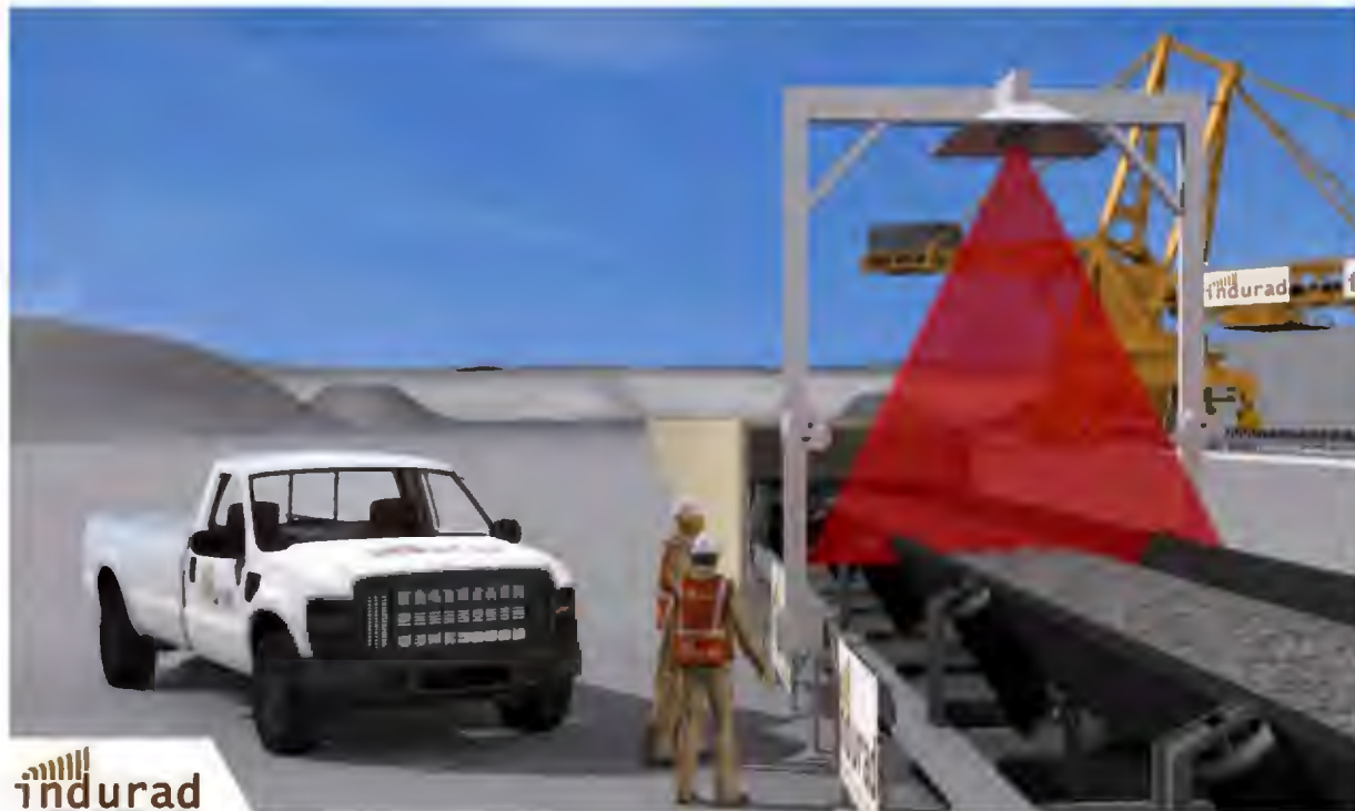
Figure 3-1: A depiction of a cross sectional area measurement device. [2]
