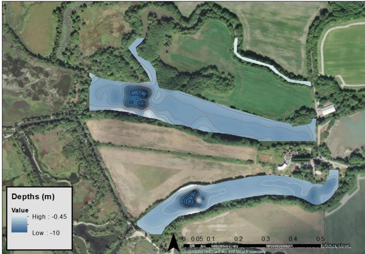
Figure 2 – The bathymetry profiles of both Ewen and Fuller Reservoirs. These maps were compiled from individual depth readings ( $n \approx 100/\text{reservoir}$ ). There are two deep (10 m) ‘pockets’ at the western ends of the reservoirs, while the remainder of the water level is around 1.5–2 m in depth.
