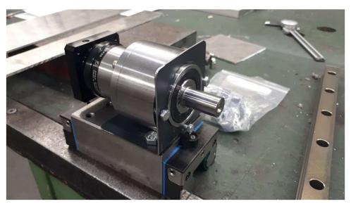
Figure 4.5 - Gearbox Mounting Bracket
