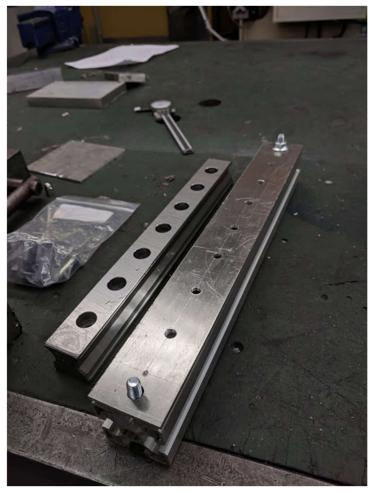
Figure 4.6 - Linear Slider T-slot Mounting
