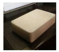
Figure 9 - Foam casting before machining
