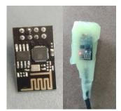
Figure 16 - Wi-fi Sensor before and after waterproofing
