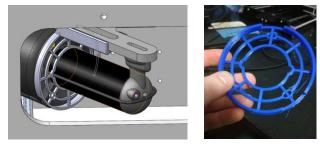
A key feature which is a requirement for passing tech are thruster guards to ensure fingers do not get sucked into the thruster. The company made custom 3D printed guards which attached semi permanently to the thruster. These thruster guards are pictured in Figure 20
