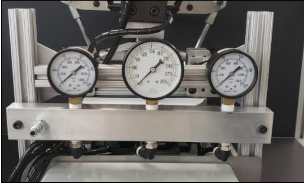
Figure 4.16 - Pressure Gauges at Back of Device
