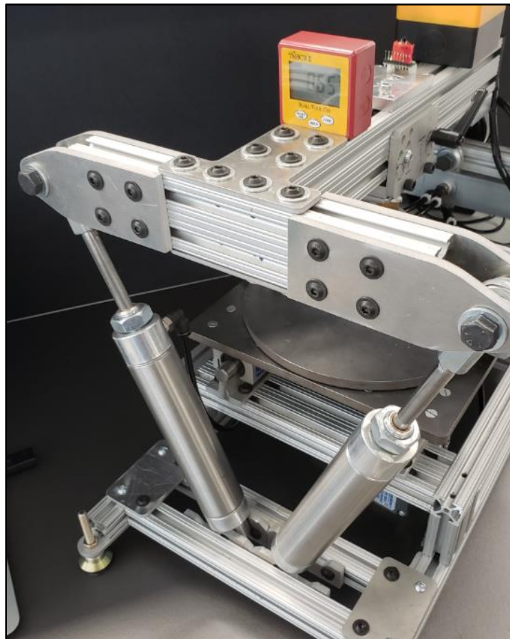
Figure 4.18 - Inclinometer for Calibration
