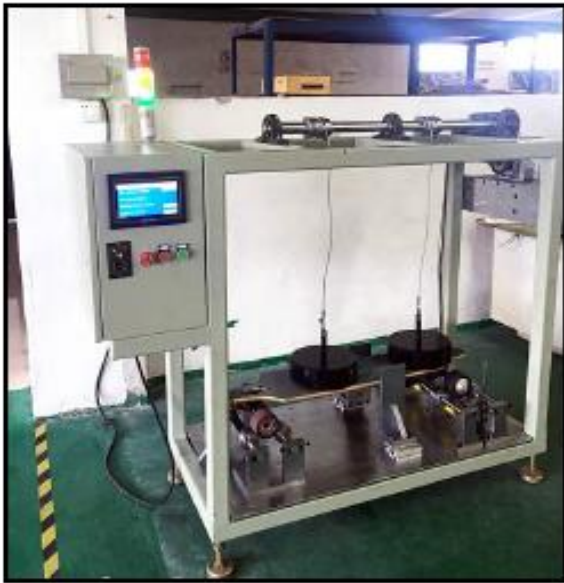
Figure 17: The ONAN Electric Skateboard Driving Simulation Device
