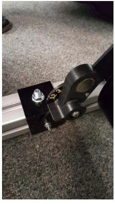
Figure 5.13 Magnet Resistance Settings
