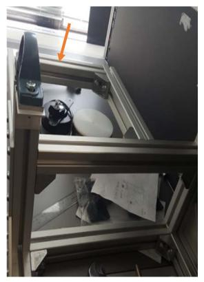
Figure 4.3 (1 x 8") Aluminum T-slot Extrusions
