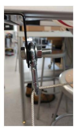
Figure 5.3 Eye Socket with Nylon Rope
