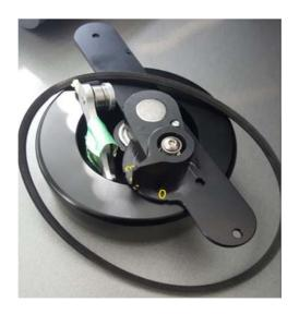
Figure 4.22 Magnetic Flywheel Assembly
