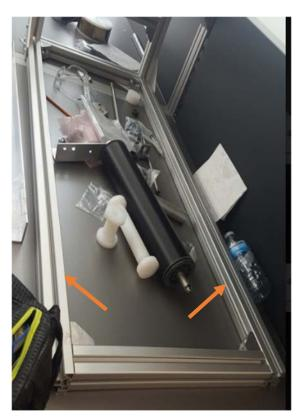
Figure 4.2 (2 x 42") Aluminum T-slot Extrusions
