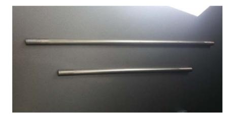
Figure 4.12 Aluminum Shafts for Bearing Blocks
