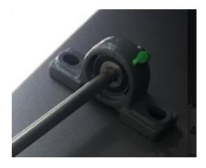
Figure 4.24 Bearing Block
