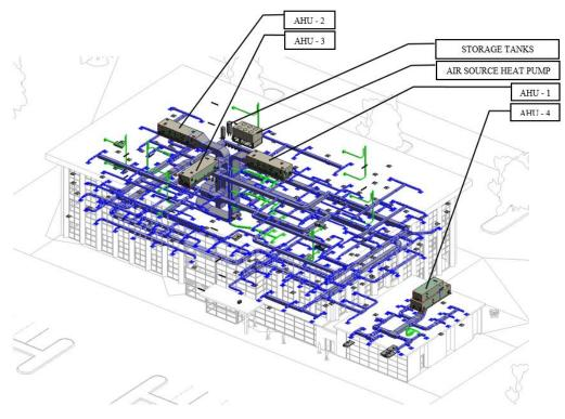
Figure 9. Duct Design
