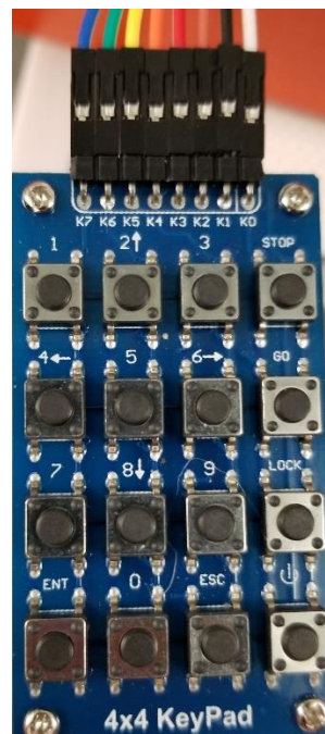
Figure 5. Keypad, numbers for mole, 4 th column for level, 4 th row for reset
