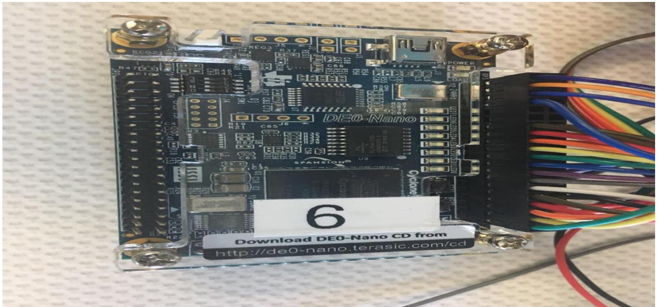
Figure 1 - Field Programmable Gate Array of 3.3V DC voltage
