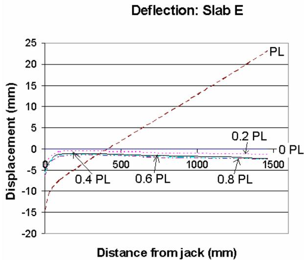
Figure 8: Deflection of WWM + Cellulose Fiber Reinforced Slab
