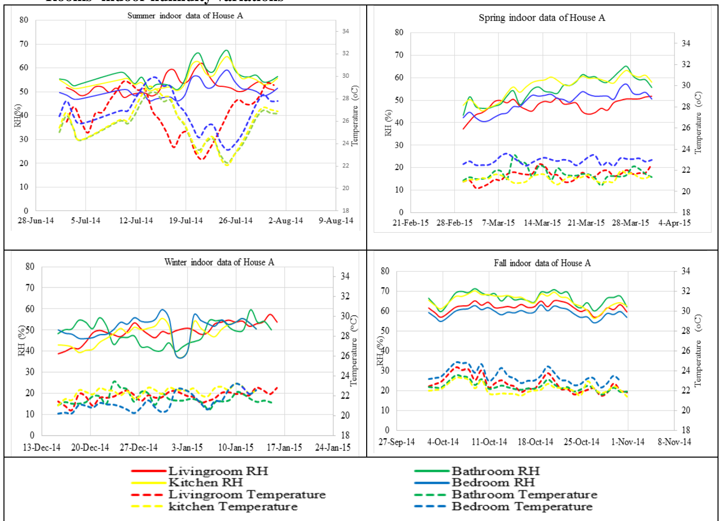
Figure 1. Indoor temperature and relative humidity of different rooms at House A
