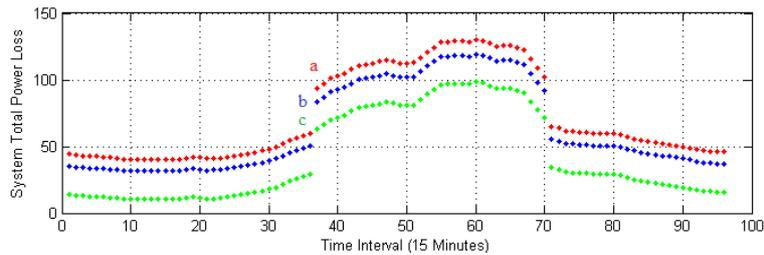
Fig. 6. System Loss Curve for Different Scenarios: a) without VVO/CVR, b) VVO/CVR confines to the substations and c) VVO/CVR implementation within substations and along distribution feeder
