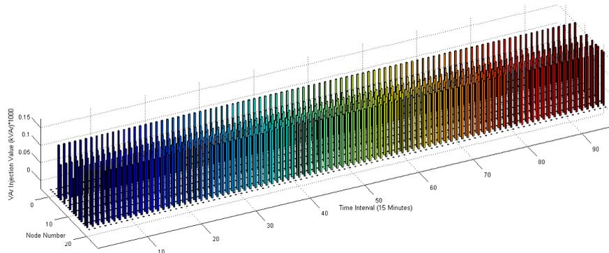
Fig. 9. CB VAR injection point candidates at each real-time interval
