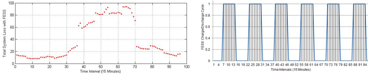
Fig. 10. The Effect of FESS on VVO/CVR and its Charge/Discharge Cycle
