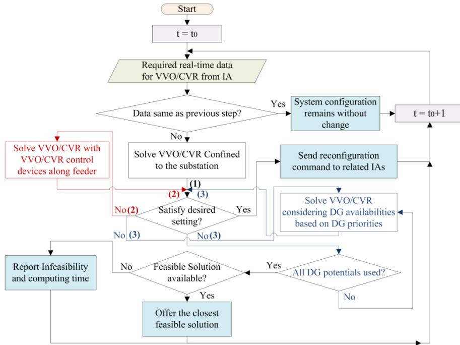
Fig. 2. Proposed real-time optimization algorithm for VVO/CVR
