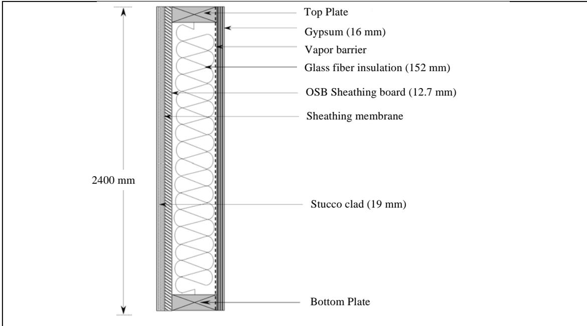
FIGURE 1: SCHEMATIC DIAGRAM OF A STUCCO-CLAD WALL CONSIDERED IN THE STUDY
