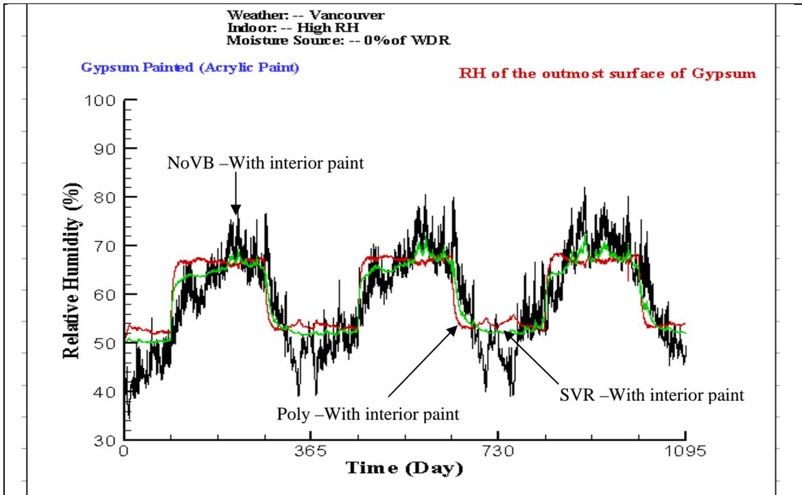
**FIGURE 6 TRANSIENT RELATIVE HUMIDITY PROFILES OF A POINT AT THE BACK OF INTERIOR GYPSUM BOARD IN DIFFERENT VAPOUR CONTROL STRATEGIES WITH SIMULATION CASES OF 0% WDR.**
