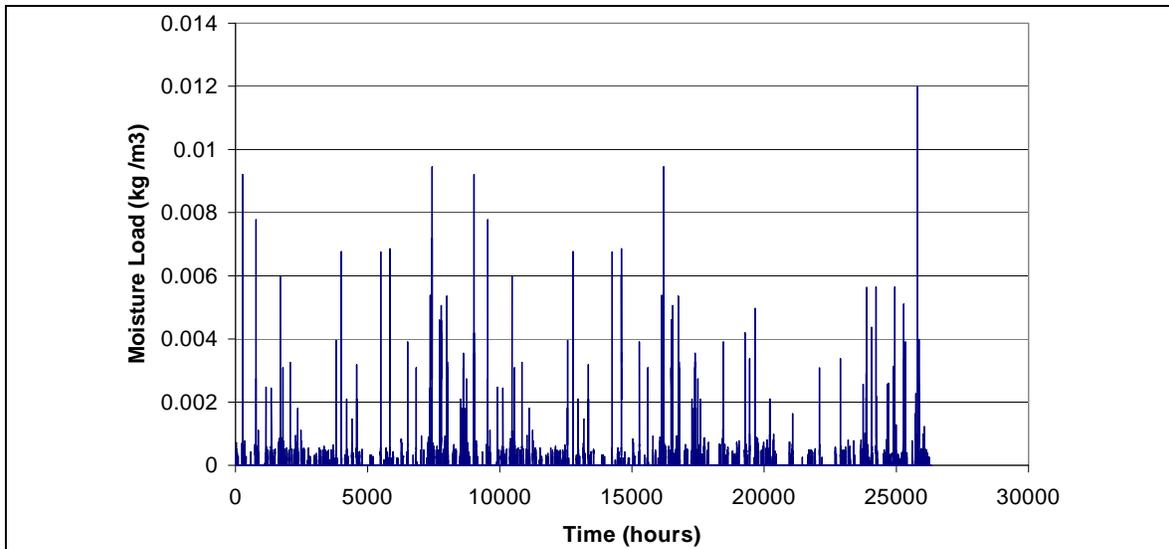
**FIGURE 3: INTERNAL MOISTURE LOAD IN THE STUD CAVITY DURING THE THREE YEARS OF SIMULATION PERIOD**
