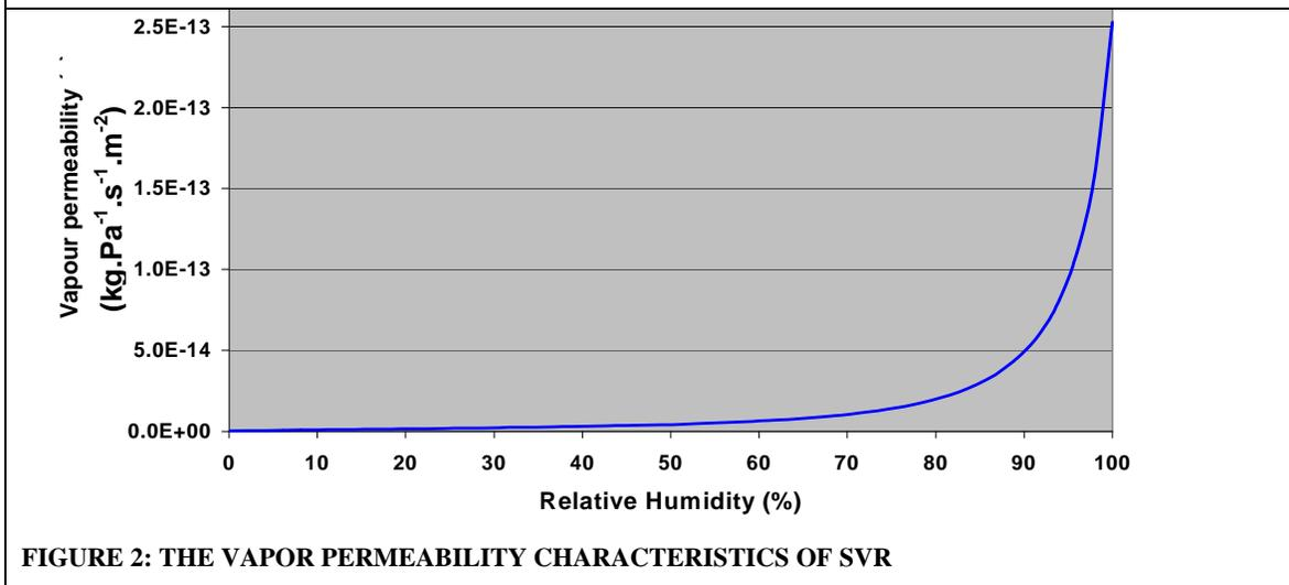
FIGURE 2: THE VAPOR PERMEABILITY CHARACTERISTICS OF SVR
