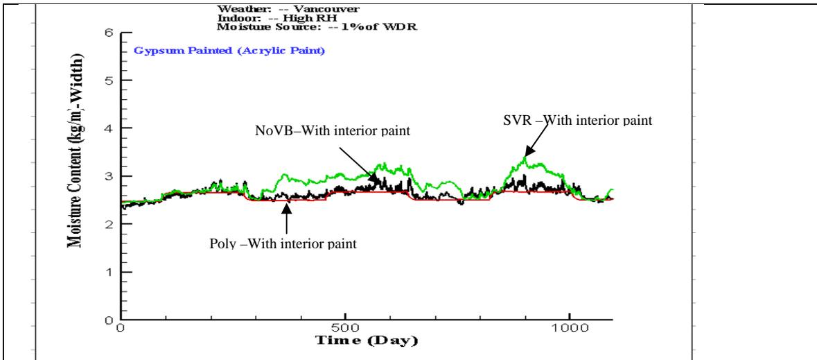
**FIGURE 8: TRANSIENT MOISTURE PROFILES OF GYPSUM BOARD IN DIFFERENT VAPOUR CONTROL STRATEGIES WITH SIMULATION CASES OF 1% WDR.**
