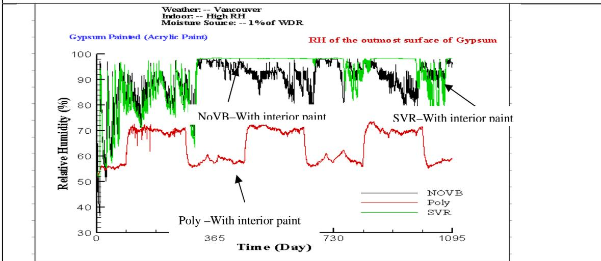
**FIGURE 9: TRANSIENT RELATIVE HUMIDITY PROFILES OF A POINT AT THE BACK OF INTERIOR GYPSUM BOARD IN DIFFERENT VAPOUR CONTROL STRATEGIES WITH SIMULATION CASES OF 1% WDR.**
