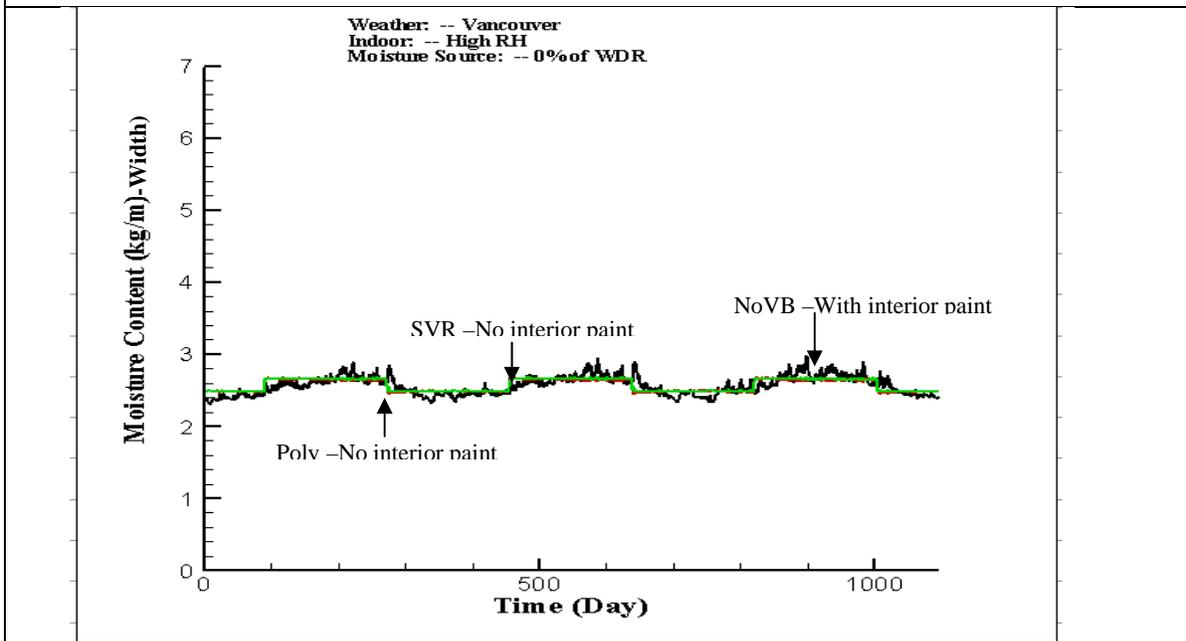
**FIGURE 5: TRANSIENT MOISTURE PROFILES OF GYPSUM BOARD IN DIFFERENT VAPOUR CONTROL STRATEGIES WITH SIMULATION CASES OF 0% WDR.**
