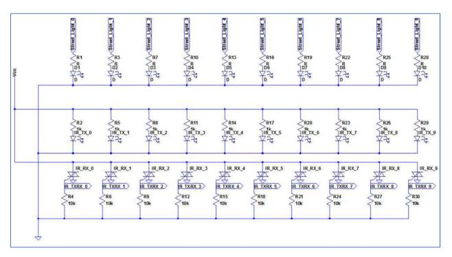
*Figure 7: Circuit diagram of the model street light system.*
