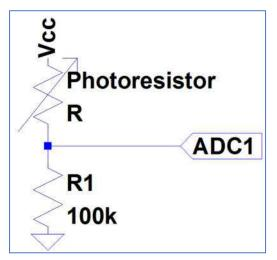
*Figure 4: Photo-resistor circuit.*
