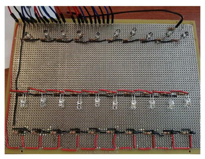
Figure 8: As-built model of the street light system containing rows of Street lights (top), IR emitter (middle), and IR receiver (bottom). V<sub>cc</sub> are the red wires, common are the black wires. Photo-resistor circuit located on top right. FPGA connections are the row of wires on the top left.
