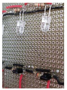
Figure 3: Infrared emitter LEDs (clear) directed at the infrared light detectors (black).
