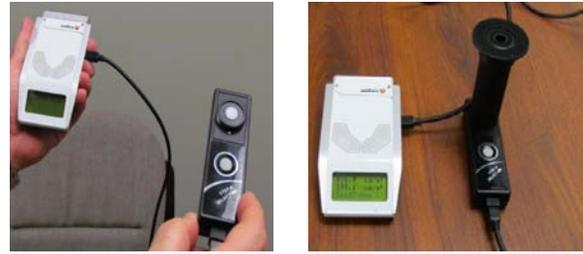
Figure 2. Light Detector without (left) and with (right) luminance tube
