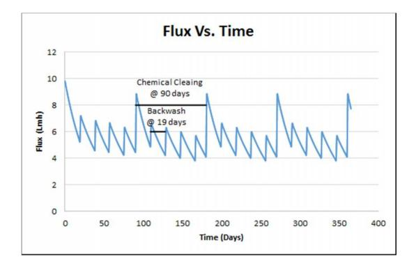
Figure 12: Optimized Backwash and Cleaning Cycle
