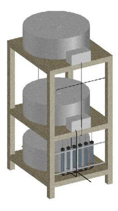
Figure 8: Isometric view of full-scale REHC treatment system
