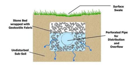
Figure 6: Concept drawing for a typical infiltration trench (Temple - Villanova Sustainable Stormwater Initiative, 2009)
