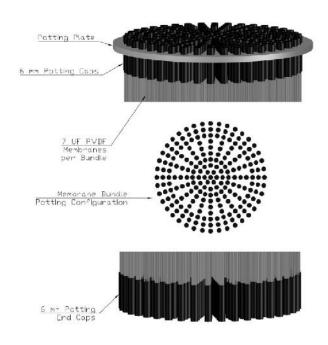
Figure 10: Membrane fibre potting configuration
