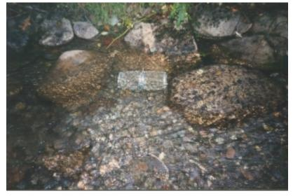
Figure 7. Gee Type Minnow Trap in Side-Channel
