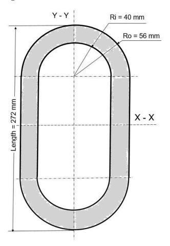
**Problem 2:** For the following cross-section determine the location (elevation) of the centroid and the moments of inertia with respect to the horizontal and vertical centroidal axes.
