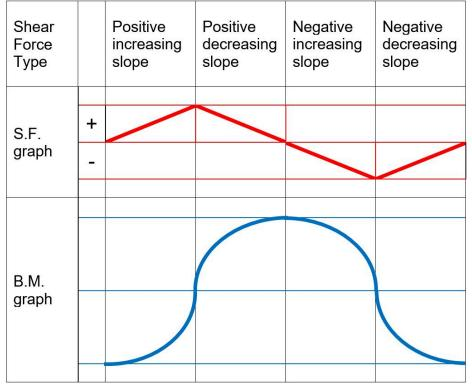
When drawing the shear force and bending moment diagrams, while the sign convention is important, consistency is crucial. For instance, consider a simple beam loaded with a point load applied on a UD load. Starting the diagrams at support A, looking towards the page, will generate the following:
