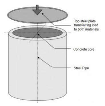
Both, the steel pipe and the concrete core work together in supporting the load therefore we must find additional relations that combine the two problems into one . Typically, we look for:
