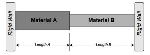
Given all the materials properties and dimensions, the objective is to calculate the stress in each section when the temperature is increased by a given  $\Delta T$ .
