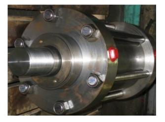
Determine the stress in the cylinder and in the tie rods. Also calculate the strain in each component using an elastic modulus of  $E_{ss} = 28 \times 10^6$  psi and  $E_{rod} = 30 \times 10^6$  psi.
