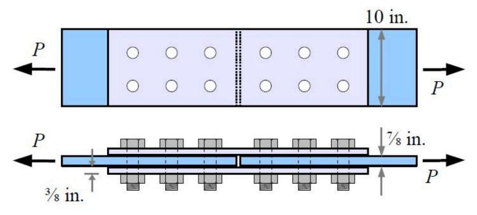
**Problem 2:** Two A36 steel plates form a lap joint with four 20 mm diameter A307 steel bolts. Calculate the maximum load that the joint can support, in kips.
