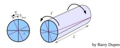
The angle of twist, [radians] is used in the general torsion equation and in estimating the shear strain,  $\gamma$  (gamma), non-dimensional.
