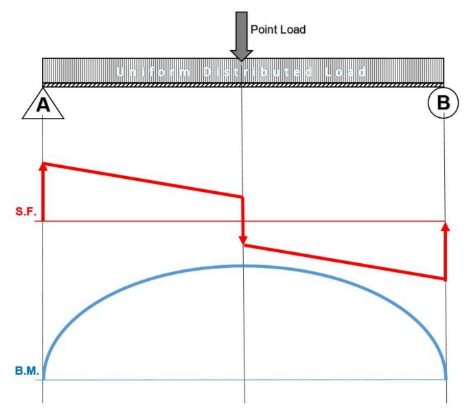
Now, flip the beam horizontally 180° (or change the observation point, looking at the beam from the opposite side) and draw the diagrams, starting from the same point A. The diagrams will appear as follows:
