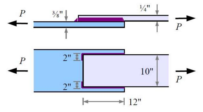
**Problem 4:** Two A36 steel plates are welded as shown with a 3/8 in. fillet weld using an E60 electrode. What is the joint strength?
