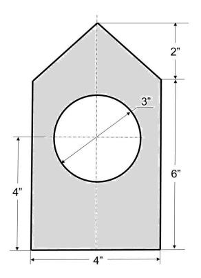
**Problem 3:** For the following figure determine Y, the vertical location of the centroid, and calculate the moment of inertia with respect to the <u>horizontal</u> centroidal axis..
