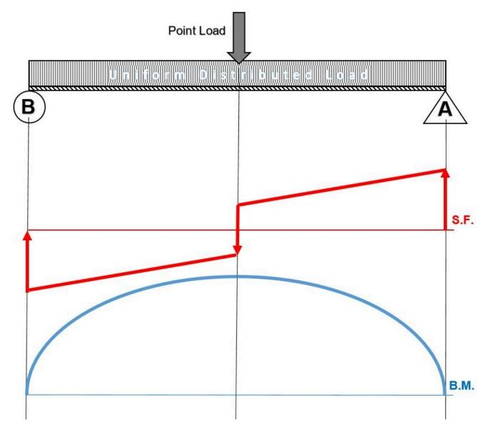
Note that, while the shear force diagrams appeared to be mirrored images (flipped horizontally), the bending moment diagram is not affected. Additionally, the most important result of this analysis, illustrates that maximum shear force and bending moment magnitudes will always be the same.
