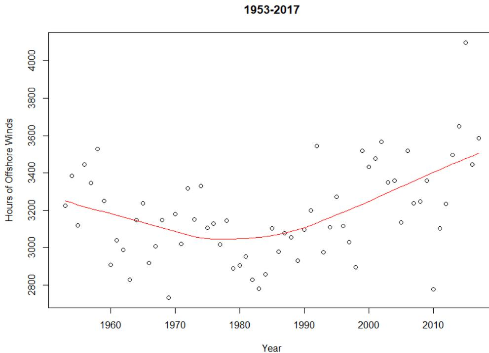
**Figure 3.2.** Graph showing the number of hourly data points recording westerly winds for each year from 1953 to 2017. Data retrieved from <http://climate.weather.gc.ca>. Line is the result of a Locally Weighted Polynomial Regression (LOWESS) fitted to these data using R Statistical Software.
