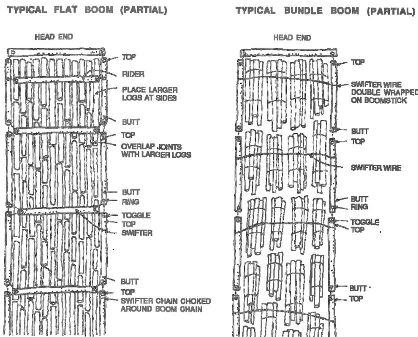
**Figure 2.13. Typical log boom construction for transportation along the BC coast (FREMP, 1991).**
