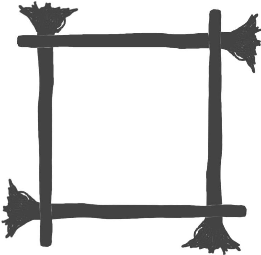
**Figure 4.8** General outline of new method for anchoring LWD structures in a foreshore environment. Anchoring is provided by root wads while the free end of each piece is fastened near the root wad of another, creating a semi-rigid structure mimicking the natural process of LWD accumulation and immobilization in the intertidal zone.
