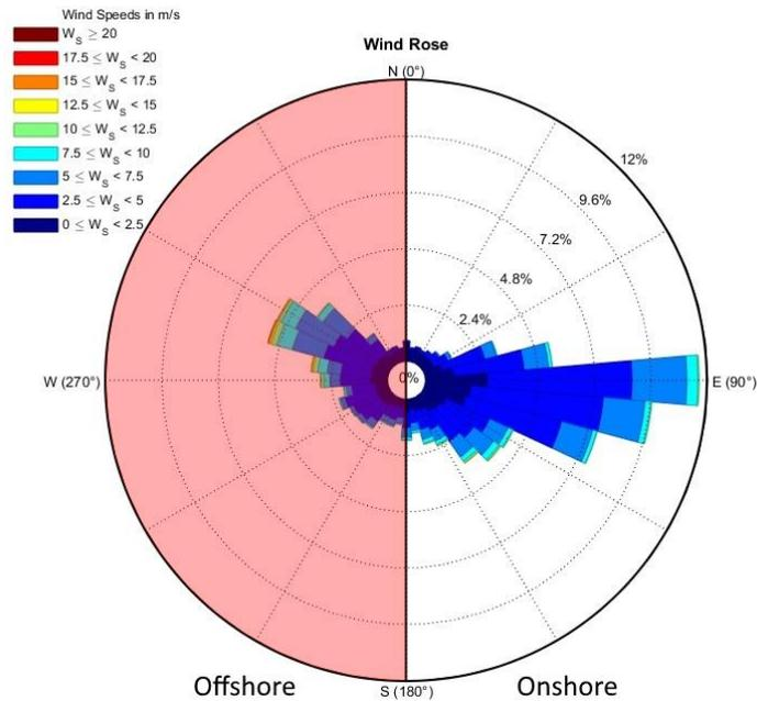
Figure 3.1 Wind rose of YVR airport between 1992 and 2012. Shaded area shows winds considered originating offshore. Data from <http://climate.weather.gc.ca> (modified from Marijnissen, 2017).
