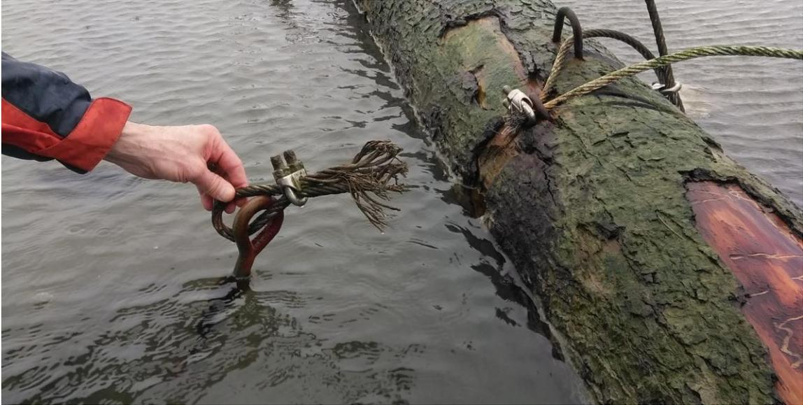
**Figure 4.6** Broken anchoring cable at plot T2, 22 March 2018. Photo by J. McDonald, 22 March 2018.
