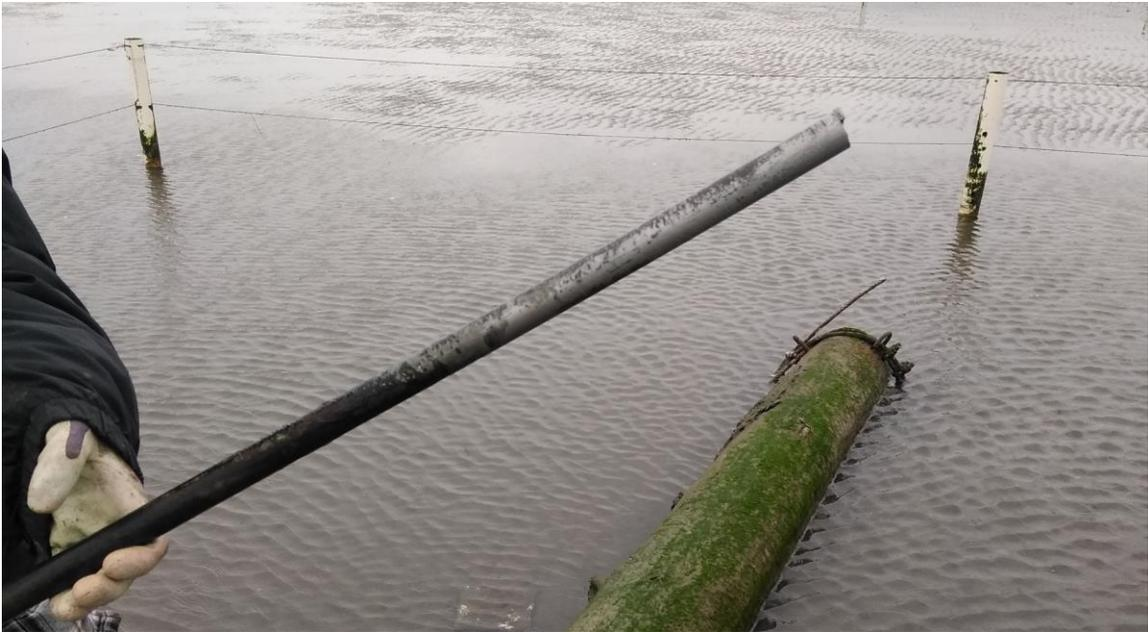
**Figure 4.7** Broken helical ground anchor at plot T3. Photo by J. McDonald, 22 March 2018.
