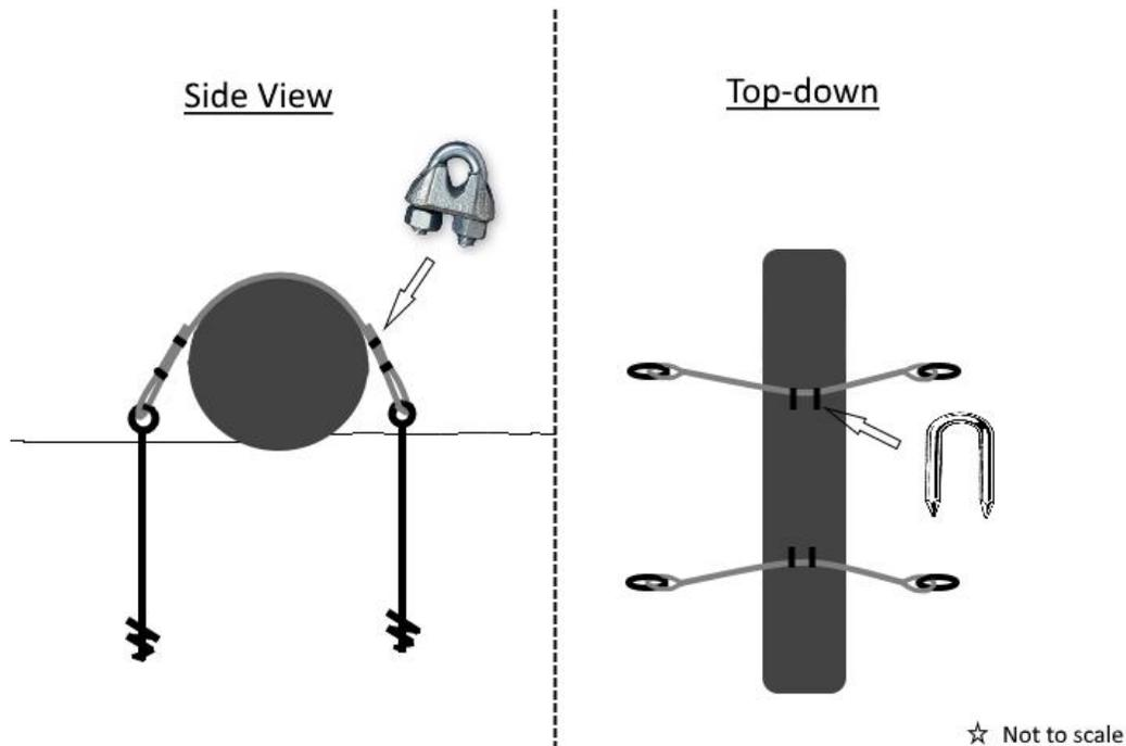
**Figure 4.3. Diagram showing installation technique used to secure LWD.**
