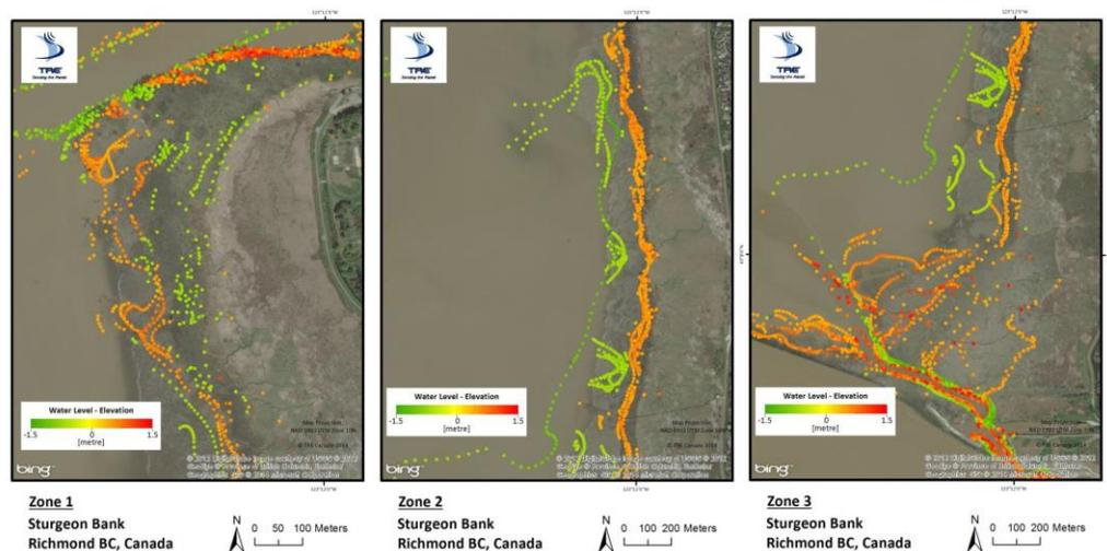
**Figure 2.10** Results of the change in surface elevation analysis over the north end (zone 1), middle (zone 2), and south end (zone 3) of Sturgeon Bank. Orange dots represent a decrease in elevation >0.5 m compared to a 2013 DEM. Green dots represent a gain in elevation >0.5 m compared to a 2013 DEM (modified from Hsiao et al., 2014).
