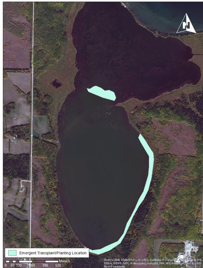
Figure 13. Proposed location of emergent transplants along the shoreline of the south basin of South Lake. Groundwater flows in a north-west direction, therefore the shoreline most exposed to polluted groundwater should be targeted (Hoole et al., 2005).
