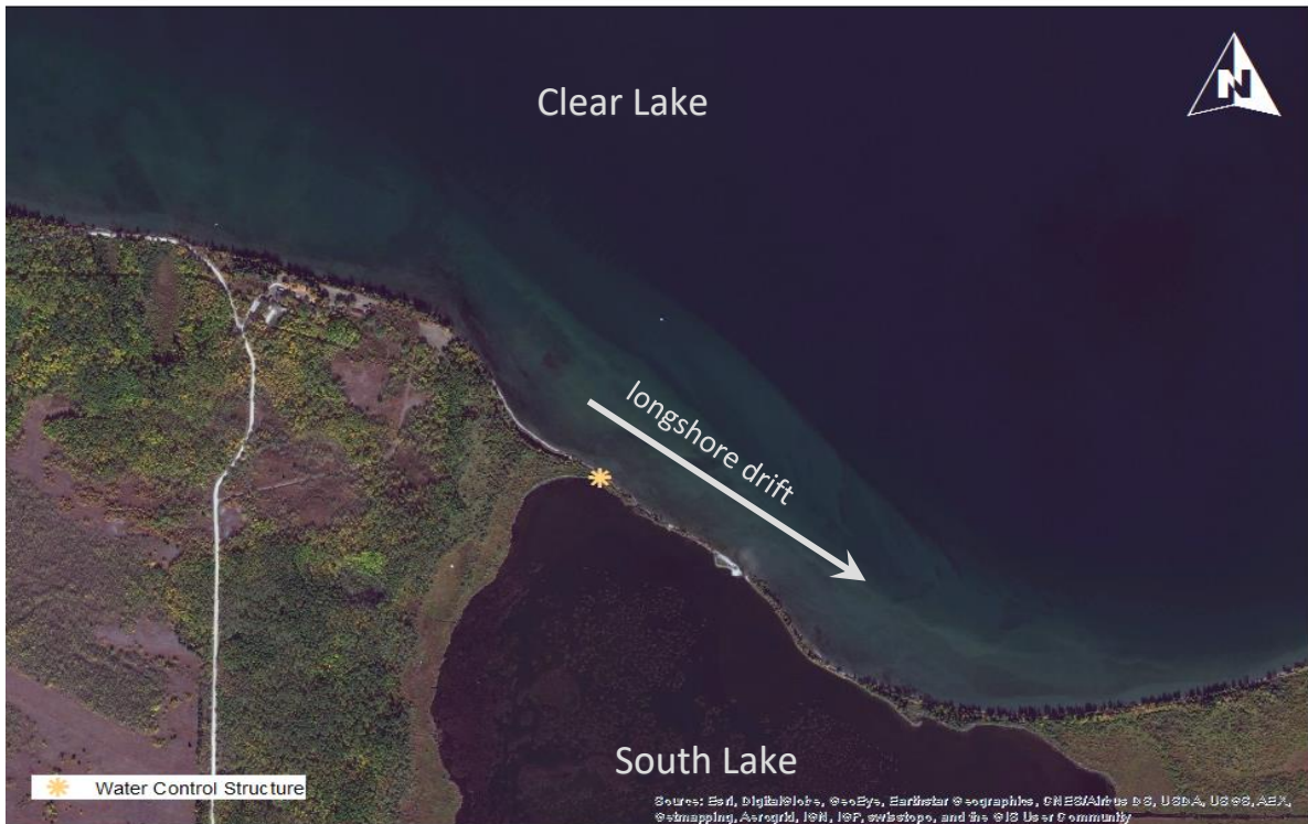
Figure 20. Proposed location of the water control structure in the isthmus. Longshore drift moves along the grey arrow in an easterly direction (Willis Cunliffe Tait DelCan, 1982).
