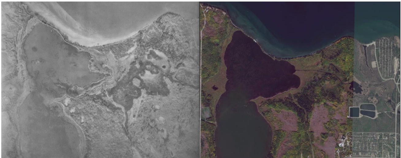
Figure 7. A comparison of a historical air photo (1966; Left) and recent satellite imagery of the north basin of South Lake (right). The constructed channel connecting Ominik Marsh and South Lake is clearly visible in the recent image.
