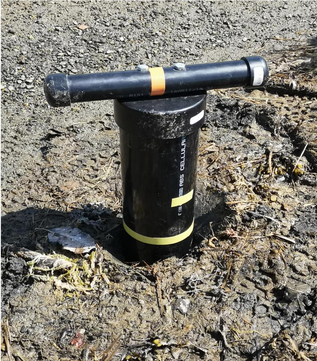
*Figure 20. Photo of PVC corer used to extract sediment containing benthic invertebrate samples and soil samples for a study done on behalf of the Nature Trust of BC during a restoration project started in 2019 at the Nanaimo estuary, Nanaimo, BC.*
