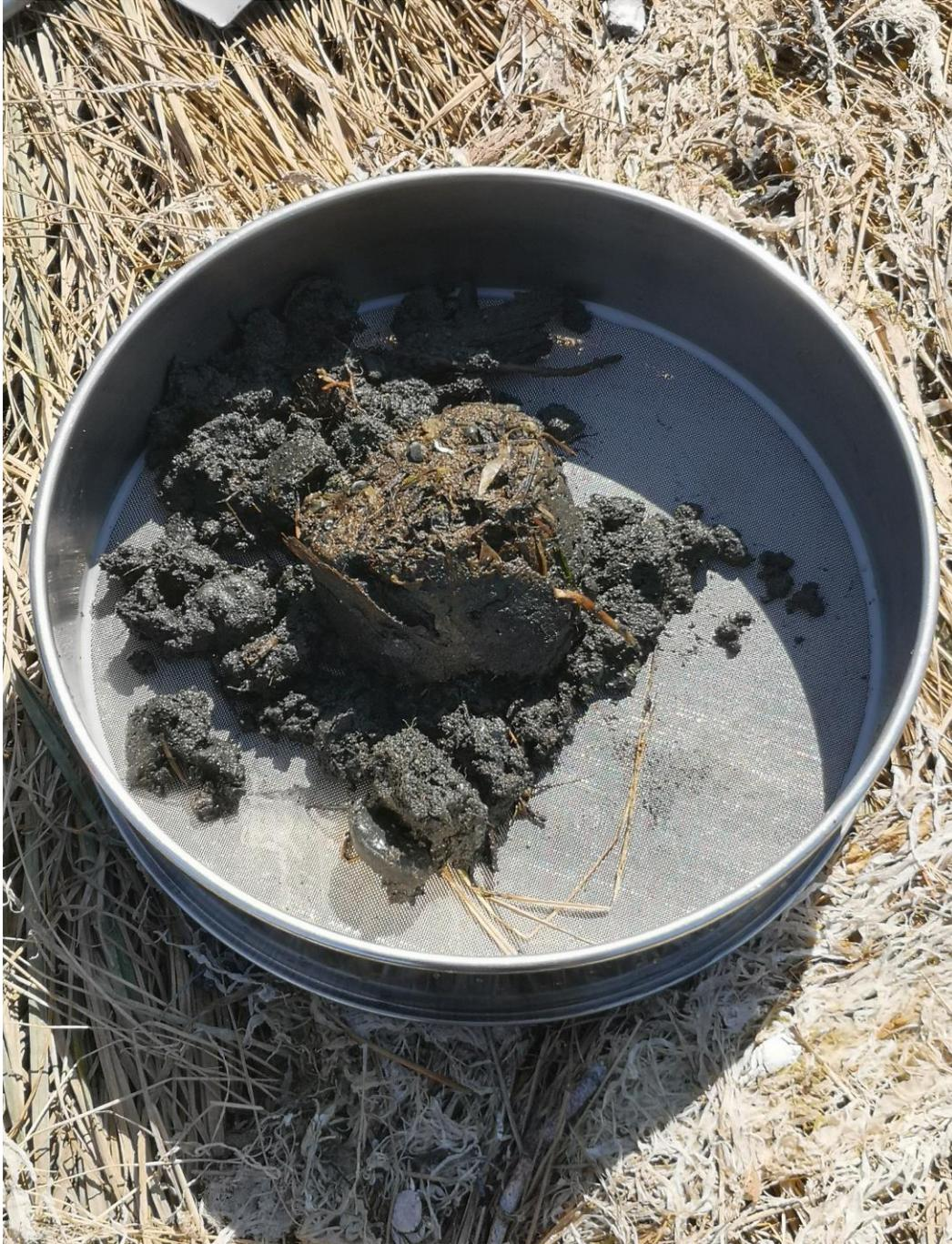
*Figure 21. Photo of a 0.5mm sieve and a typical soil core extracted for benthic invertebrate samples and grain size analysis for a study done on behalf of the Nature Trust of BC during a restoration project started in 2019 at the Nanaimo estuary, Nanaimo, BC.*
