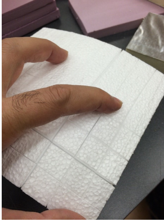
Figure 6-8. A grid of cuts on one side of EPS samples for sorption test.
