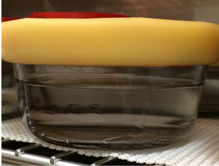
Figure 6-22. A sample wet cup filled with distilled water to 15 mm below the specimen.
