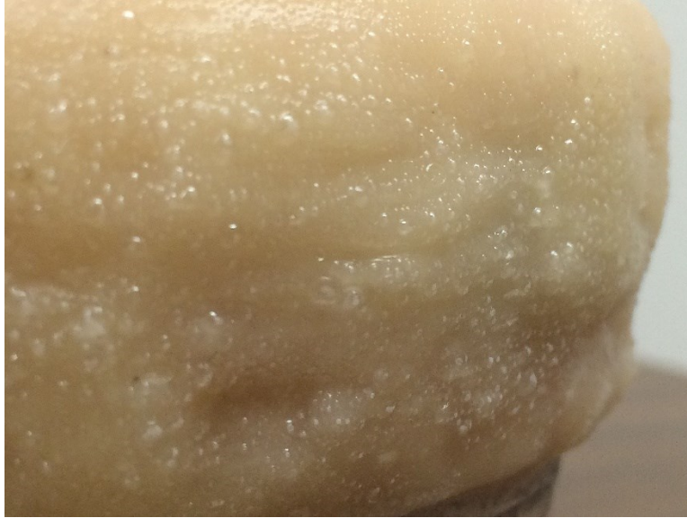
Figure 6-21. Melted normal wax mixture with air bubbles at temperature 45°C.
