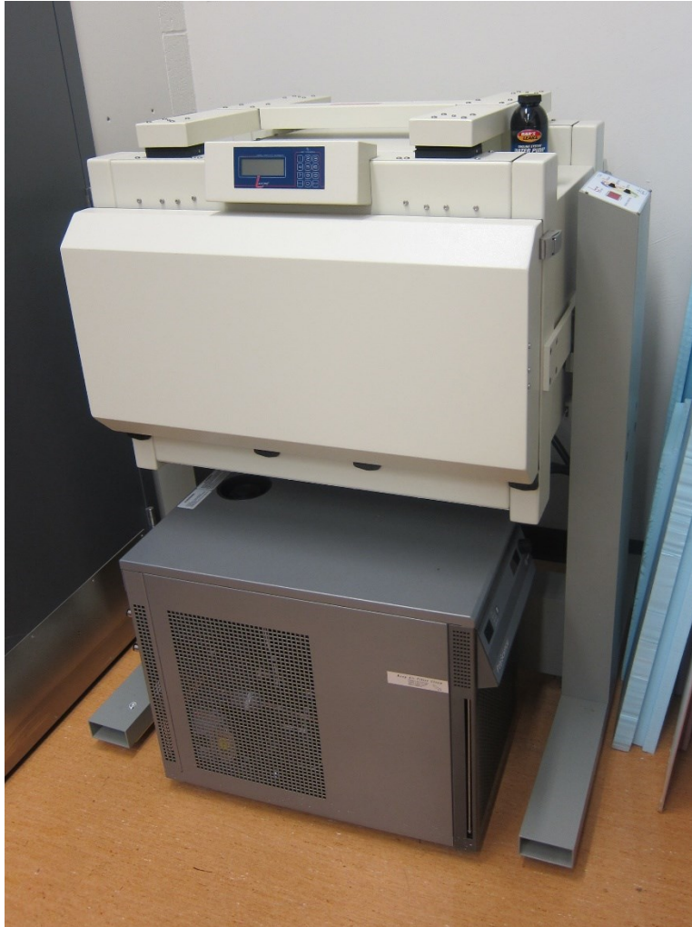
Figure 6-7. The LaserComp Fox 600 HFM in the material lab at BCIT center of excellence.
