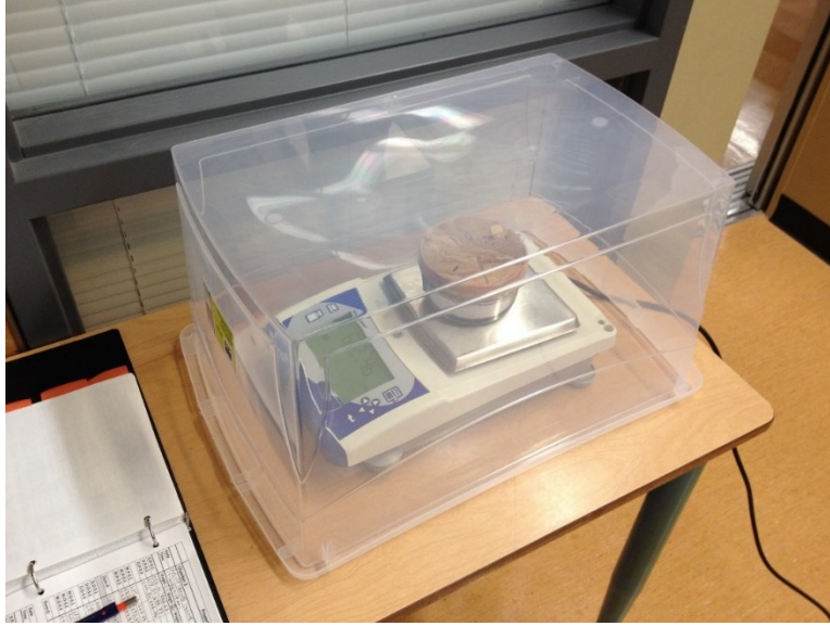
Figure 6-31. Electric balance with the accuracy of 0.01 g and a clear cover box.
