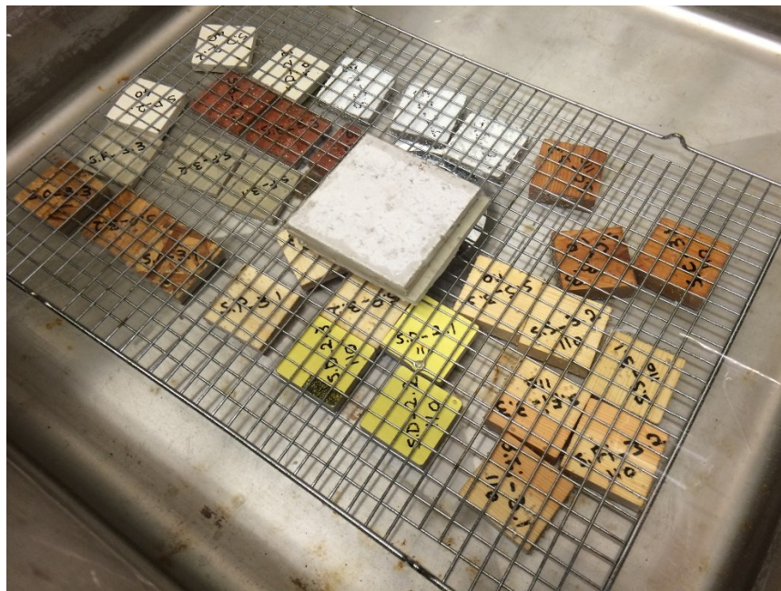
Figure 6-17. Specimens were kept under at least 15 cm of water for 8 days to reach full fiber saturation equivalent.
