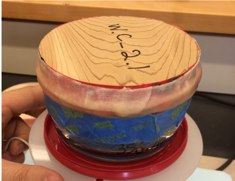
Figure 6-24. The joint between the specimen and the cup is reinforced by using a band gauze.
