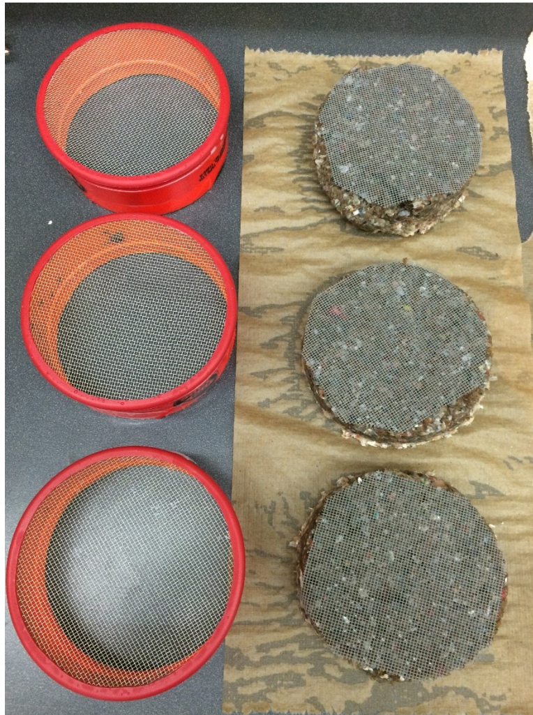
Figure 6-35. A cylindrical plastic frame with a stainless-steel mesh was made for the water absorption test of cellulose fiber samples.
