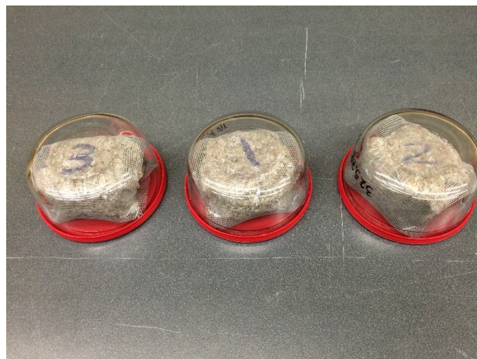
Figure 6-14. The cellulose fiber samples wrapped by a plastic mesh and kept in containers.
