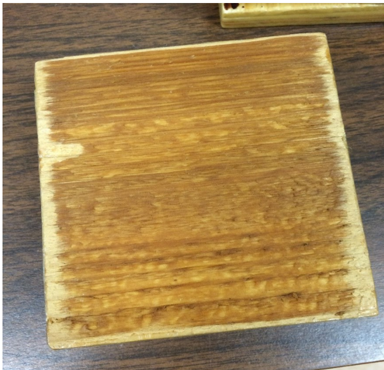
Figure 6-34. The penetrated wax into the wood fiber limited absorbing water through the full area of the surface.
