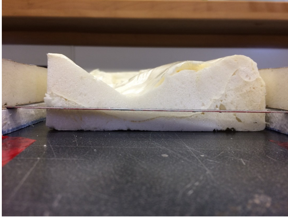
Figure 6-5. Rough and uneven surfaces were removed on the samples of sprayed foam insulation.
