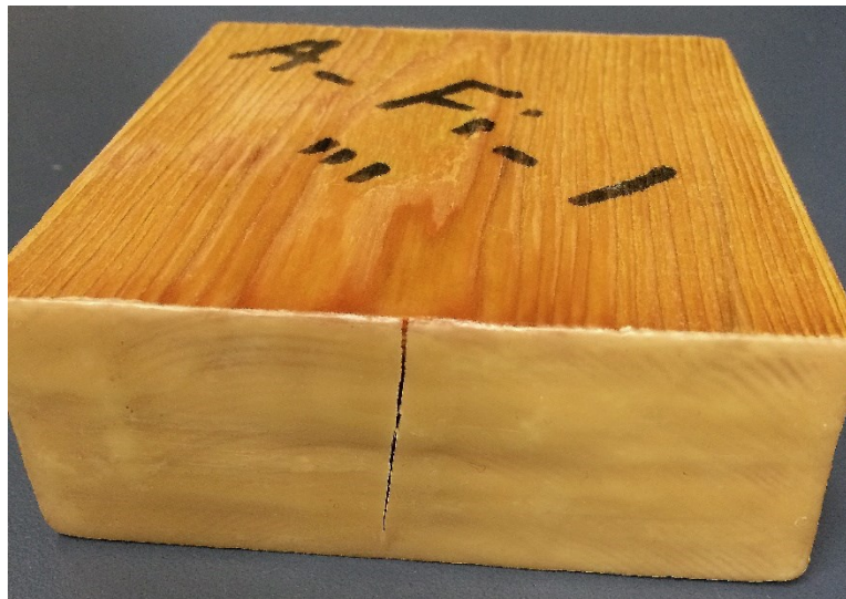
Figure 6-32. A crack in wax sealing even with gauze reinforcement on a Douglas fir sample during the water absorption test.
