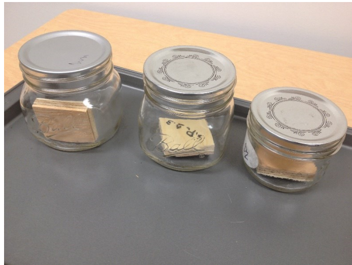
Figure 6-13. The plywood specimens inside the airtight glass containers during the weighing process.
