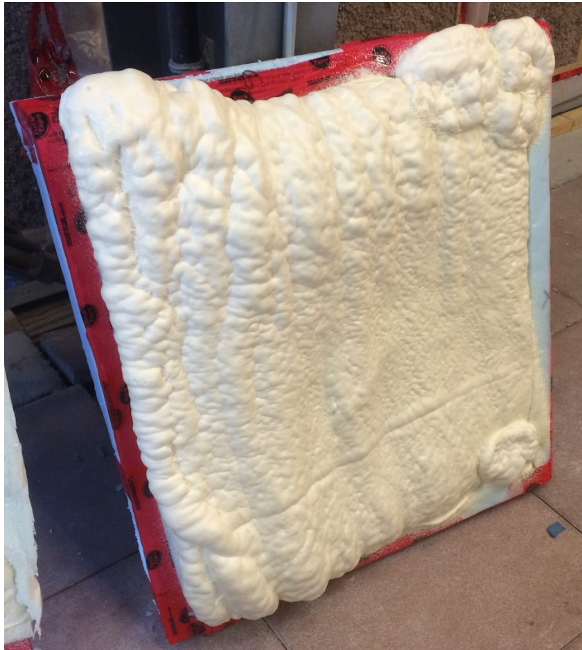
Figure 6-4. Sprayed foam insulation samples with rough and uneven surface.
