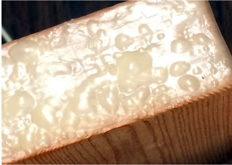
Figure 6-33. The normal mixture wax melted during water absorption test at 45°C.
