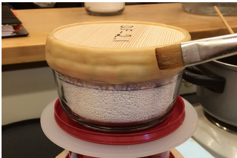
Figure 6-25. Sealing the specimen on the cup with applying wax mixture.
