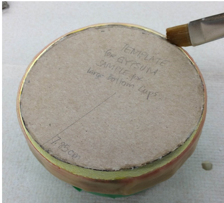
Figure 6-26. During sealing test cups, the top surface of the material samples was protected by a cardboard template.
