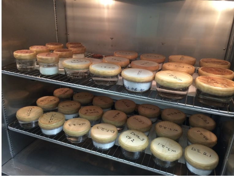
Figure 6-29. Dry and wet cup samples inside a climate chamber.
