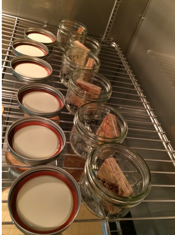
Figure 6-15. The OSB and plywood specimens remained in the open containers while exposed to the condition inside the climatic chambers.
