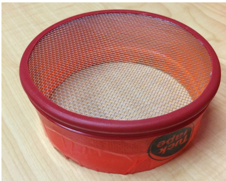
Figure 6-27. A plastic cylindrical frame with stainless-steel mesh on one side.
