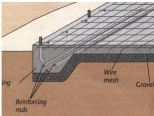
Figure 2: Image obtained from Concrete Network (2019) of slab on grade foundation.
