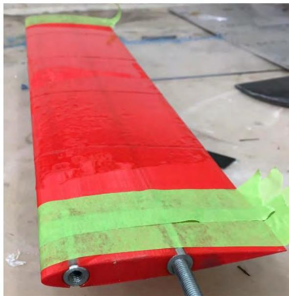
*Figure 3.33: 3D printed mast core with aluminum connecting rods.*
