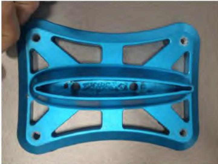
Figure 11: Cabrinha pedestal for joining the mast to the board.
