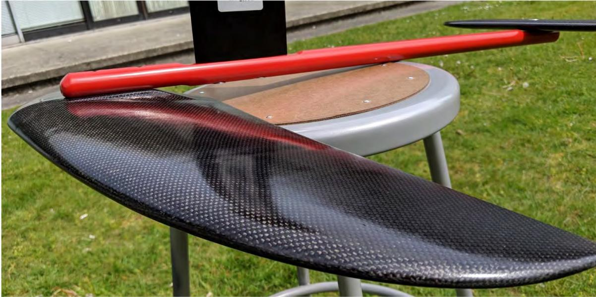
*Figure 3.25: Front wing with clear coat and top coat applied.*
