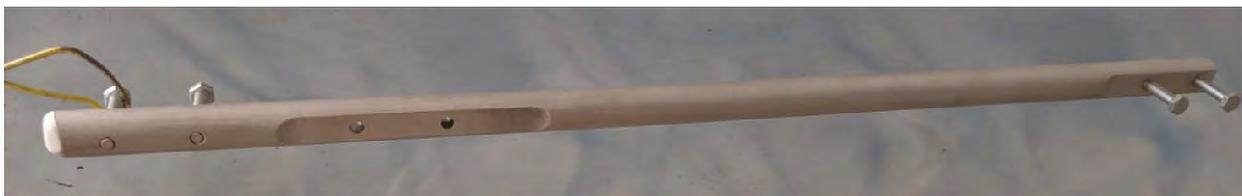
*Figure 3.31: Fuselage with Rounded Profile & Sandblasted Finish*
