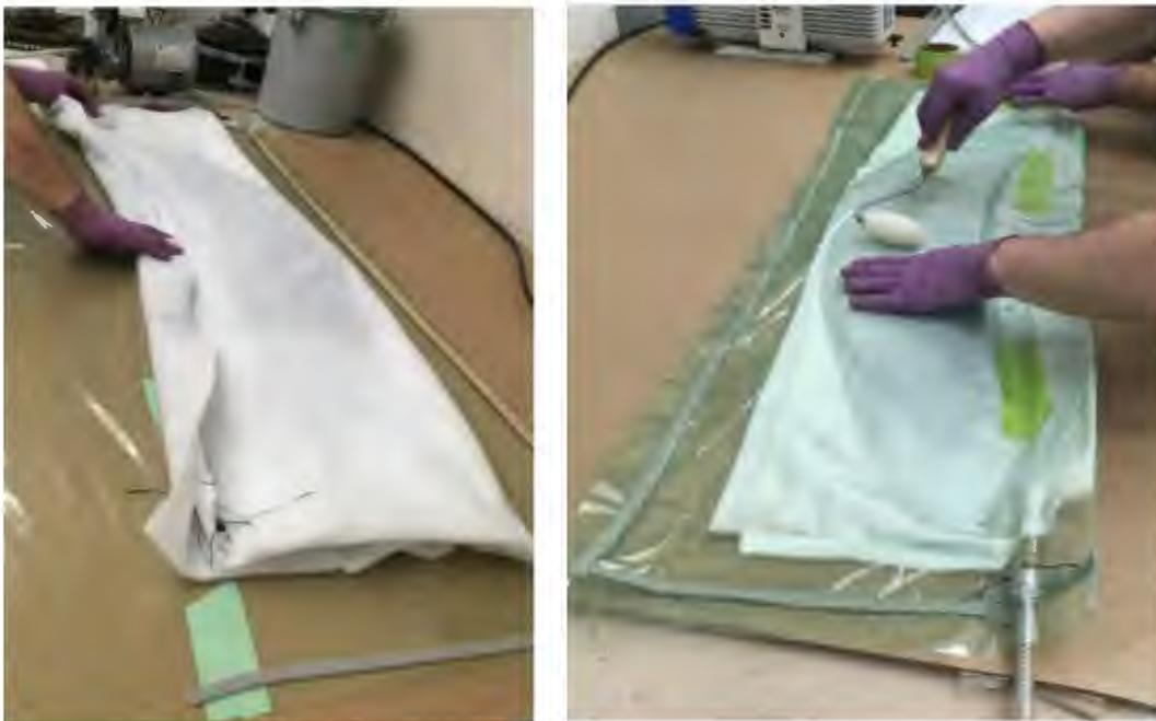
*Figure 3.24: (L) Wing Wrapped in Breather Cloth (R): Wing sealed in the vacuum bag.*
