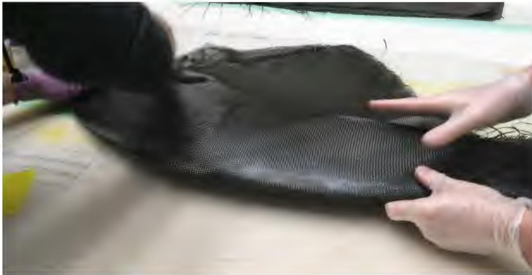
*Figure 3.22: Application of the First Carbon Fiber Layer to the Epoxied Wing Core*
