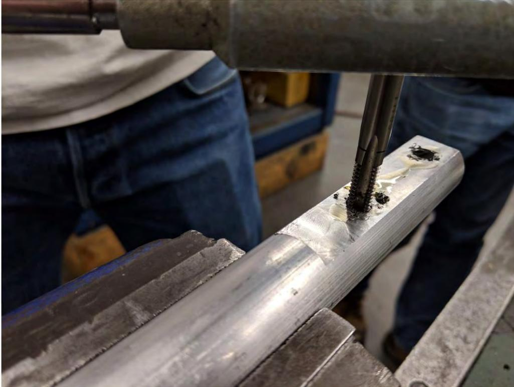
*Figure 3.30: Tapping Operation for Wing Attachment Holes*
