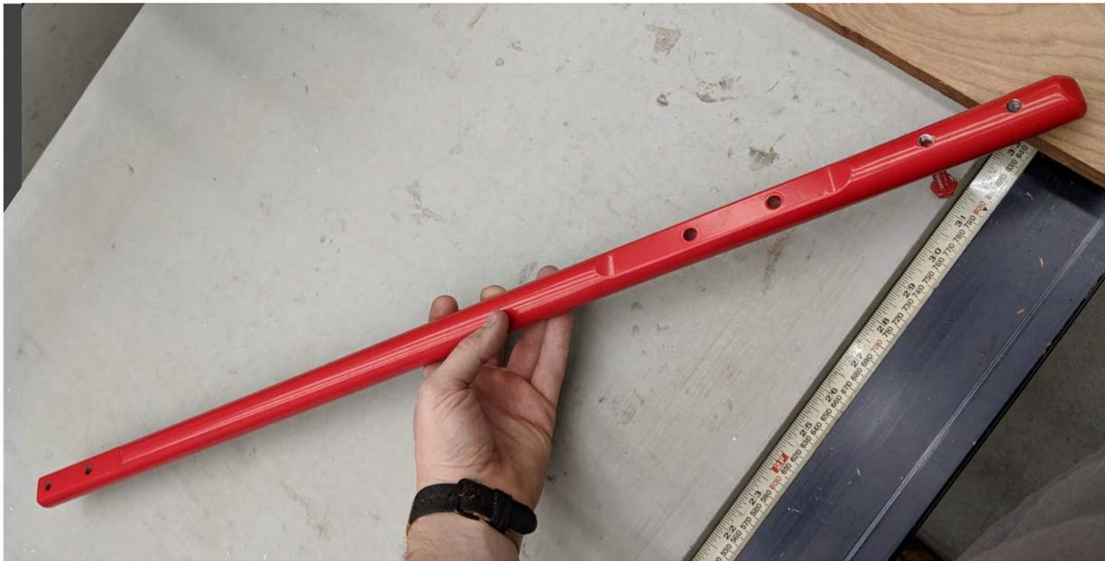
*Figure 3.32: Fuselage with Powder Coating*
