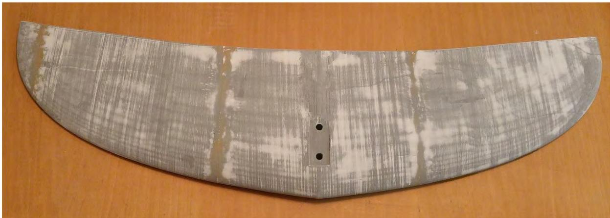
*Figure 3.20: Prototype Wing Epoxied Together, Drywall Putty Applied, & Sanded*
