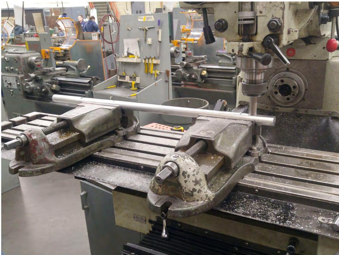
*Figure 3.26: Aluminum Fuselage Fixed in Vices on Milling Machine*
