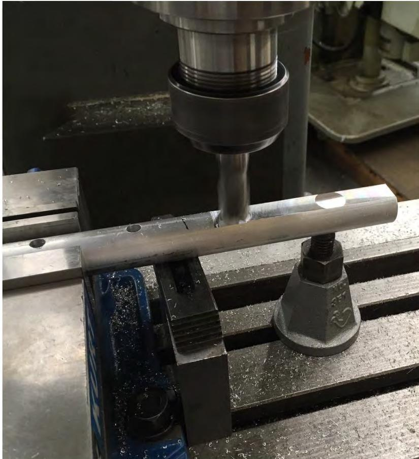
*Figure 3.28: End Mill Removing Material from Fuselage*
