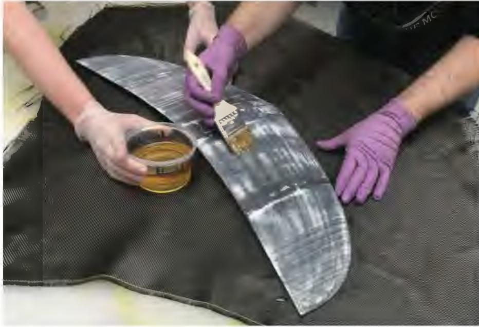
*Figure 3.21: Application of Epoxy to the Front Wing Prototype*
