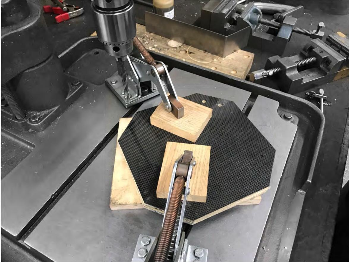
Figure 5.7. Sandwich Composite during the Drilling Process
