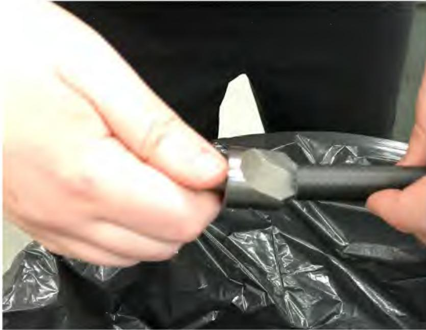
Figure 5.11. Deburring the Carbon Fibre Tubes
