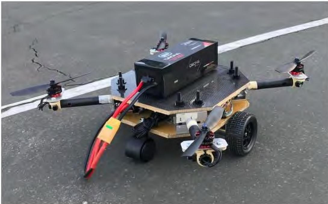
Figure 6.1: Final Hybrid Drone Concept
