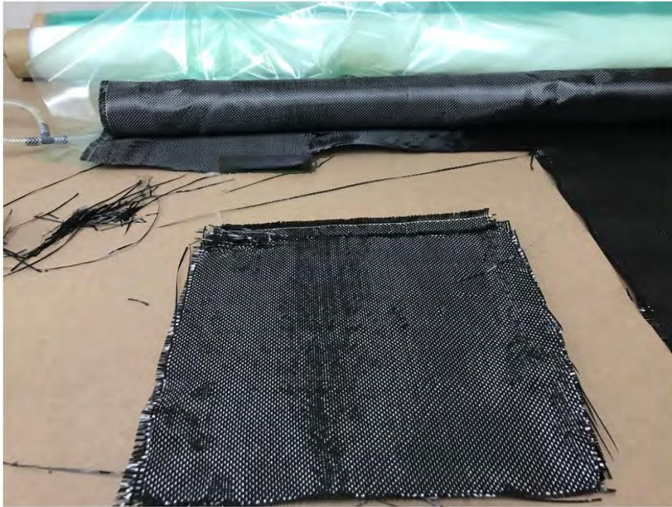
Figure 5.2. Carbon Fibre Squares
