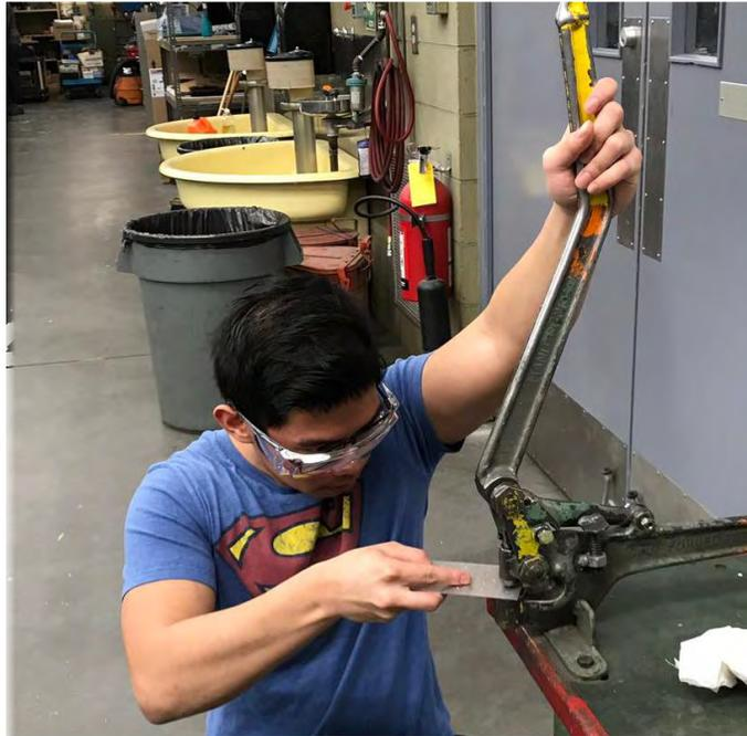
Figure 5.14. Punching Holes into the Propeller Motor Mount Parts
