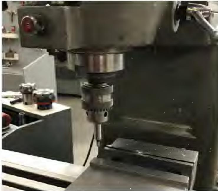
Figure 5.9. Milling Machine with Edgefinder
