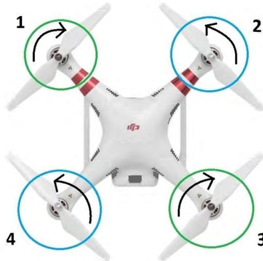
Figure 4.19: Basic Quadcopter Configuration [50]
