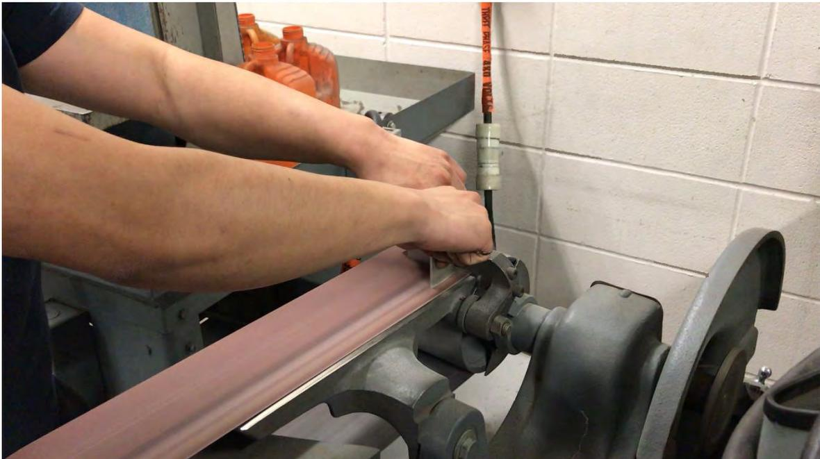
Figure 5.18. Removing Excess Material Using a Sanding Machine
