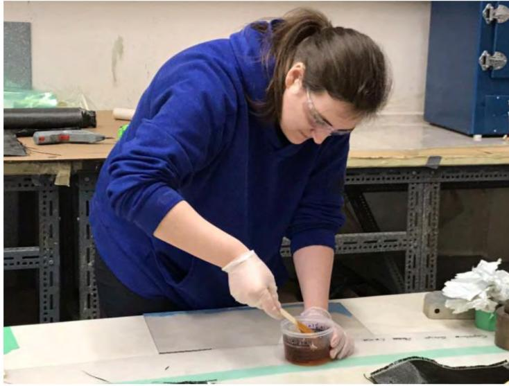
Figure 5.4. Mixing Epoxy Resin
