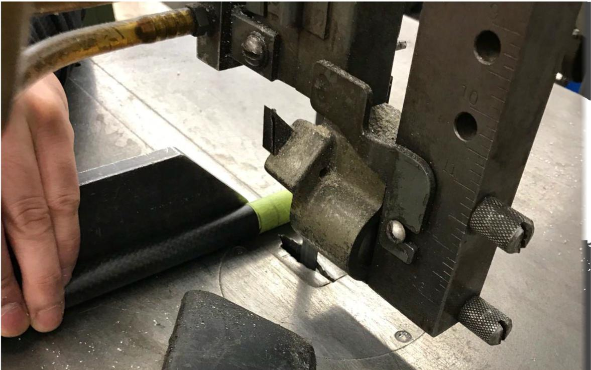
Figure 5.8. Cutting of the Carbon Fibre Tubes
