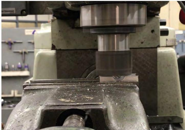
Figure 5.16. Removing Material from the Tube Clamps
