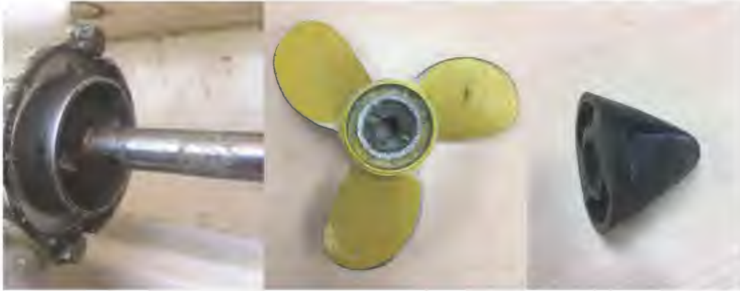
Figures 1,2,3. Propeller drive housing and shaft, propeller assembly, and retaining nut
