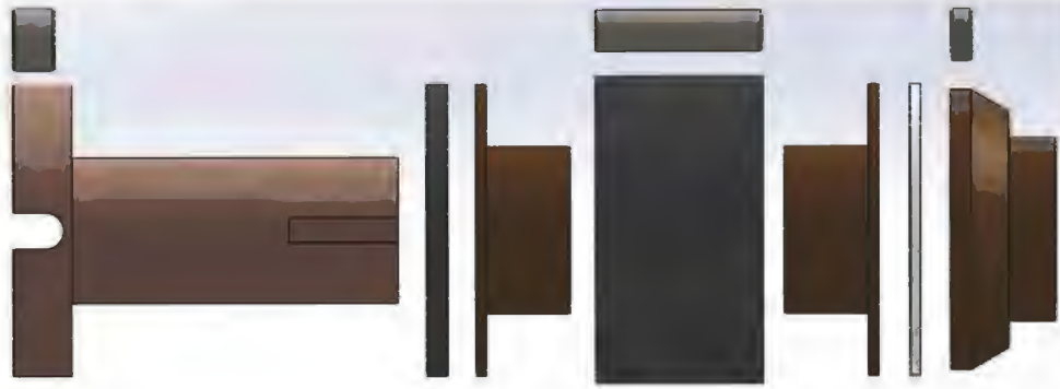
Figure 7. Exploded view. From left to right: main drive sleeve with forward magnet, friction lining, bronze sleeve, rubber bushing with center magnet, bronze sleeve, plastic layer, and rear magnet support with rear magnet.
