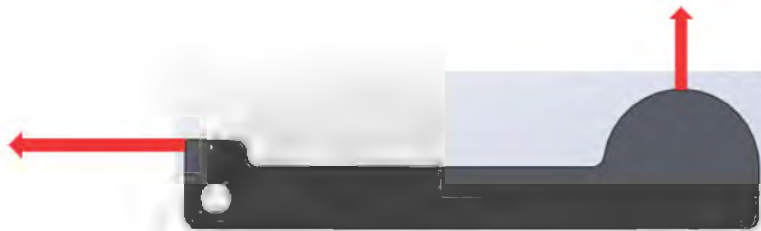
Figure 4.3.3.2 Arm with forces
