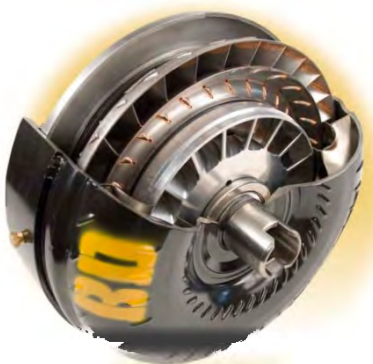
Figure 4.3.3.3 Cut-away view of a torque converter [14]
