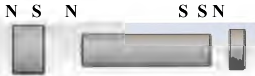
Figure 11. The polarities of one set of three magnets, and the spacing between them
