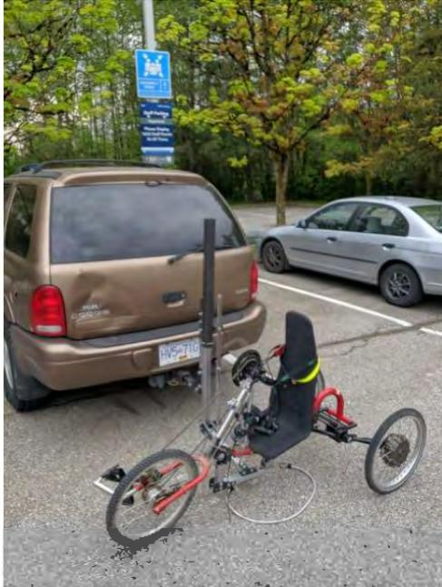
*Figure 20- side view of rack mounted on client's vehicle*
