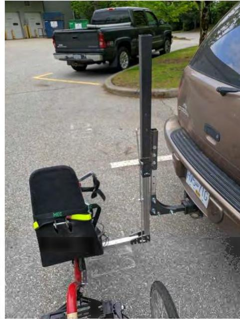
*Figure 21- view of handcycle mounted to frame on client's vehicle*
