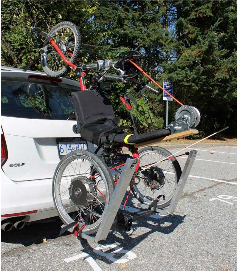
*Figure 1- previous design of clients handcycle car rack*
