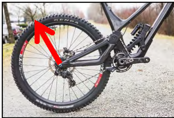
Figure 1.1 High Pivot Suspension [1]
