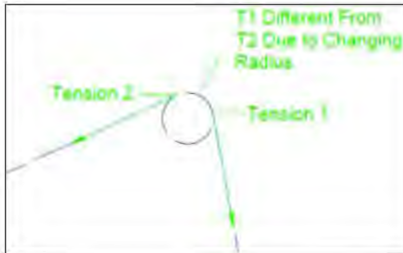
Figure 2.2 Free Body Diagram of Idler Sprocket
