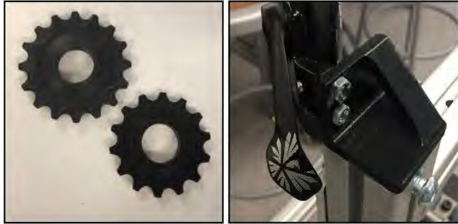
Figure 4.7 3D Printed Sprockets (left) and Shifter Mount (right)
