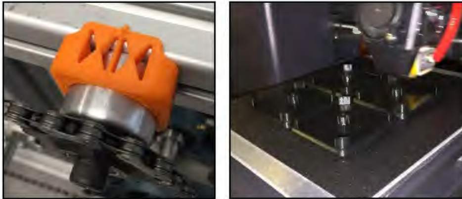
Figure 4.8 3D Printed Center Marker (left) and Extrusion End Caps (right)
