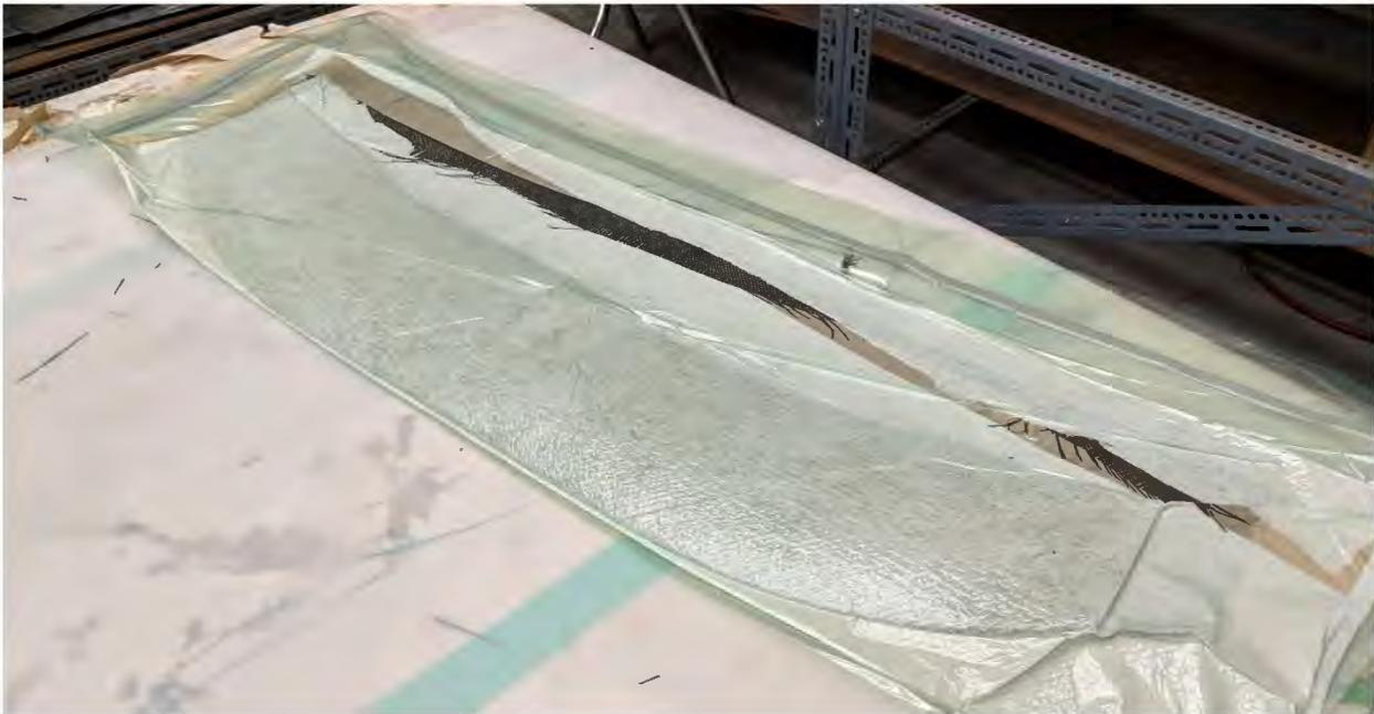
Figure 32: Vacuum bagging wing
