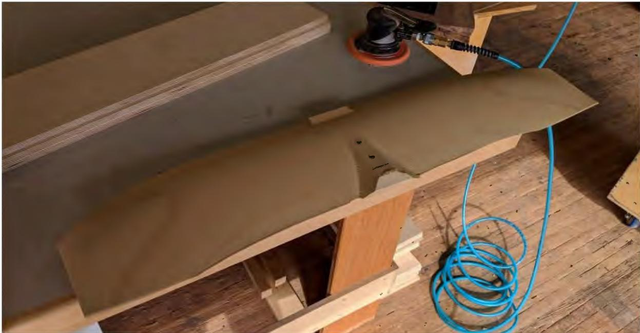
Figure 29: Wing core removed from stock piece
