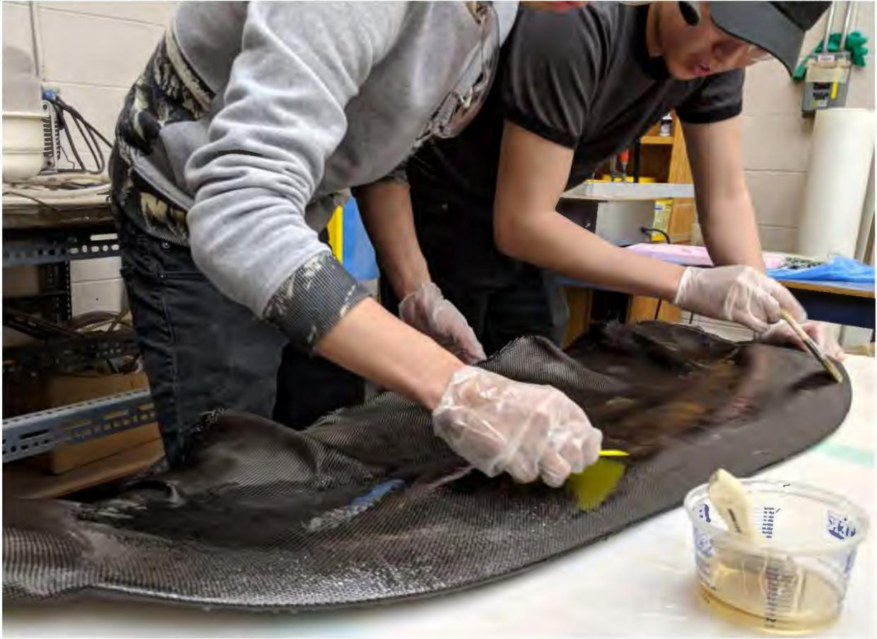
Figure 31: Carbon fiber layup process
