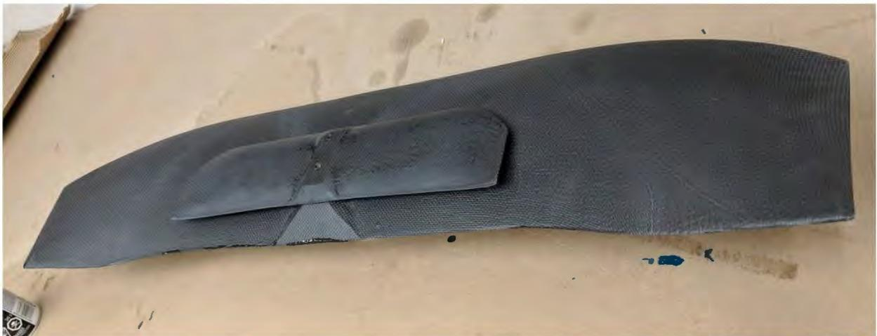
*Figure 34: Hydrofoil after excess material removed*
