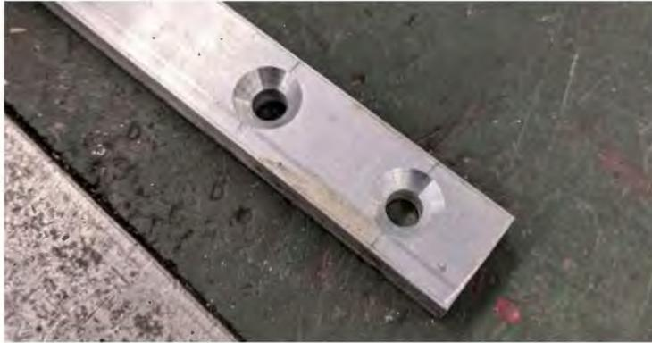
*Figure 36: Drilled and countersunk connection holes*
