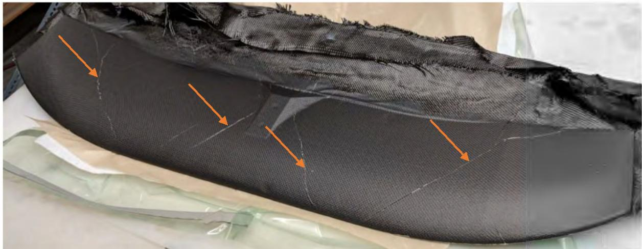
*Figure 43: Folding on carbon-fiber layer*
