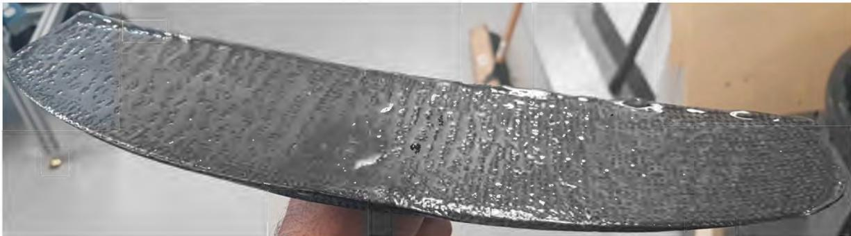
Figure 44: Non-uniform Epoxy Layer
