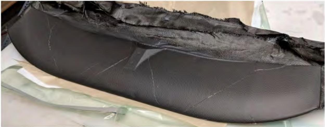
*Figure 33: Wing after vacuum bagging*
