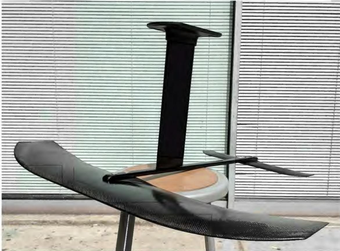
*Figure 39: Assembled Hydrofoil design*
