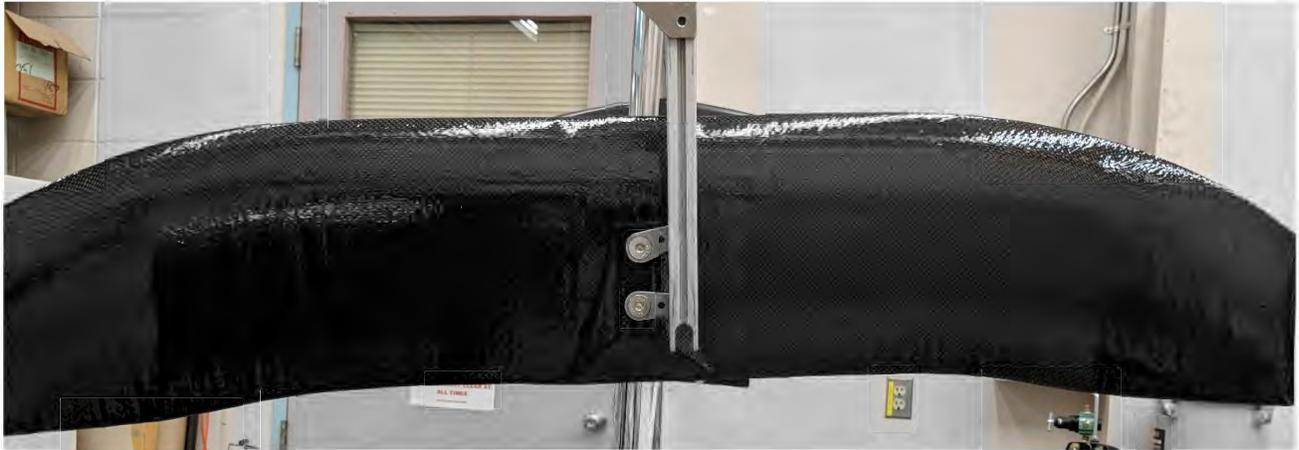
*Figure 35: Exterior coating of epoxy added*
