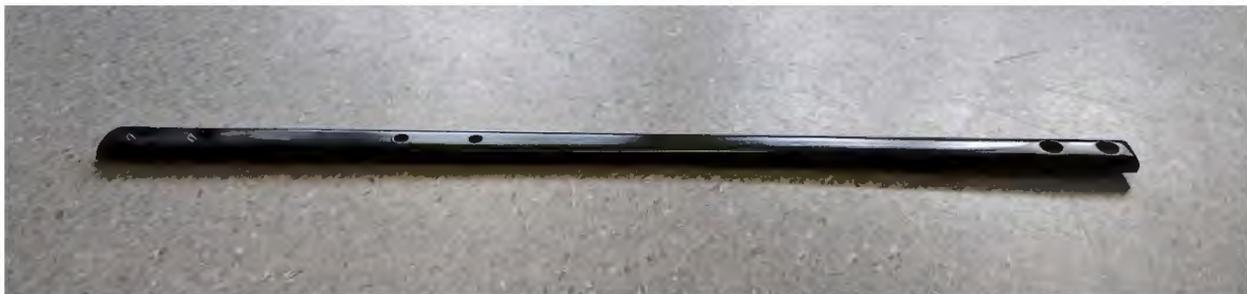
*Figure 38: Powder coated fuselage*
