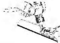
Lift the tucked-under tape end of the assembly, and, holding in the same position, apply one or two drops of M-Bond 200 adhesive at the fold formed by the junction of the tape and specimen surface. This adhesive application should be approximately 1/2 in [13 mm] outside the actual gage installation area. This will insure that local polymerization that takes place when the adhesive comes in contact with the specimen surface will not cause unevenness in the gage guideline.
