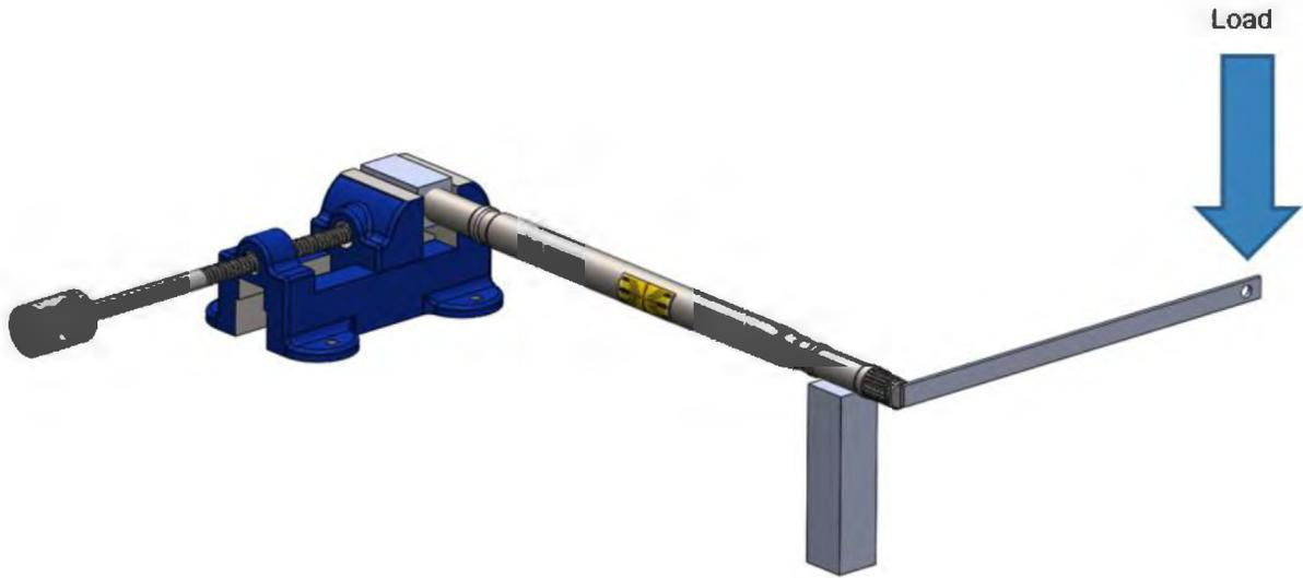
Figure 26: Torsion Test Rig
