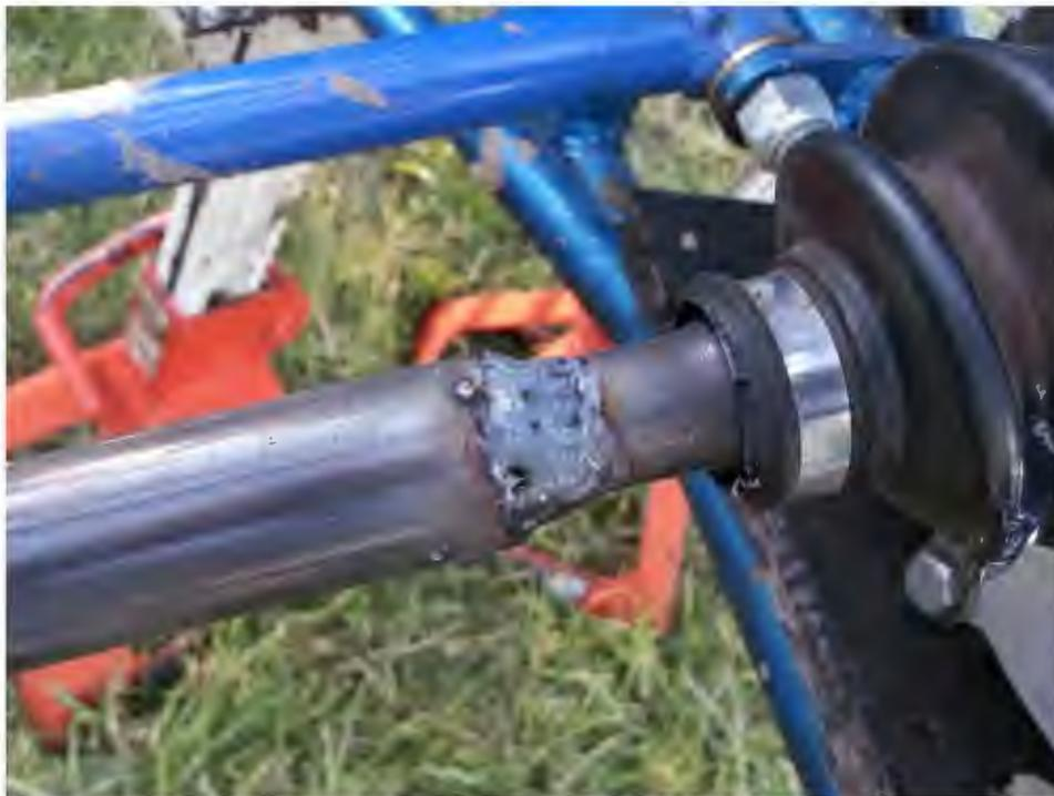
*Figure 7: Field Repair of Failed Weld on V1 Axle in Rochester, 2016*
