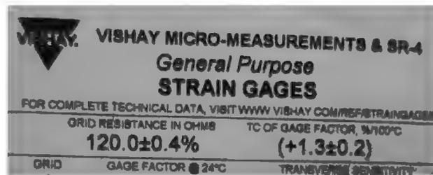
Figure 38: Strain Gauge Data Label
