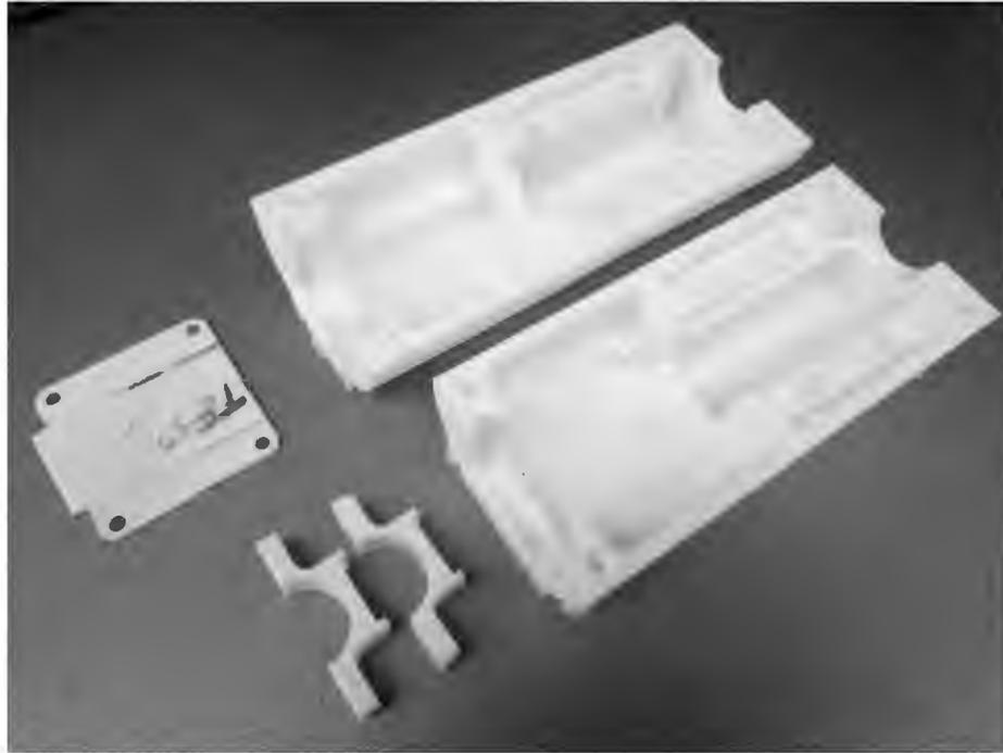
*Figure 23: Housing Design Iterations with Test PCB and Clamps*
