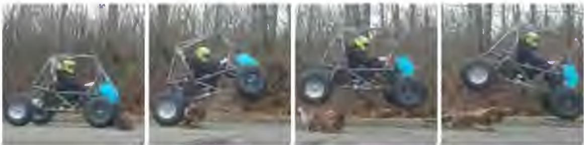
Figure 11: Destructive Testing of BCIT Racing Baja Vehicle V2, 2019
