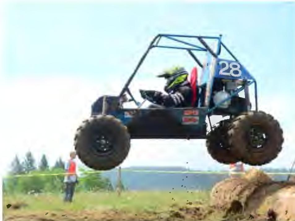
Figure 5: Moments Before Gearbox Failure Due to Impact in Oregon, 2015
