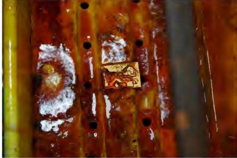
*Figure 35: PCB in Etching Tank*
