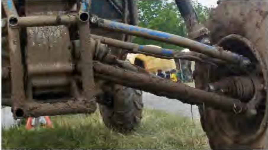
*Figure 8: Full Failure of VI Axle Shaft in Rochester, 2016*
