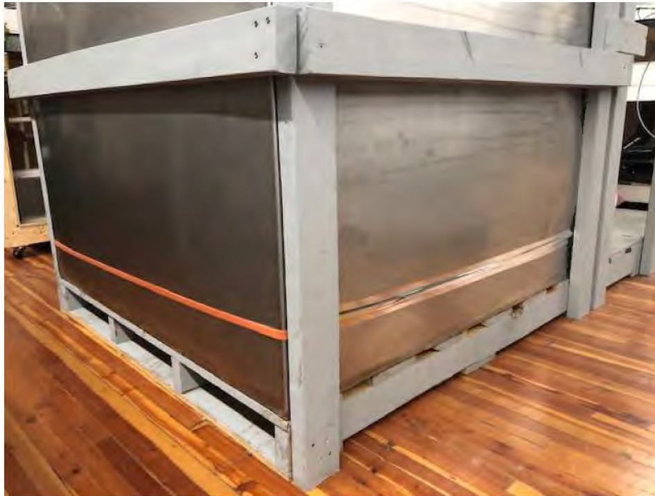
Figure 4.4 - Ground heat simulation using a 400W heat belt.
