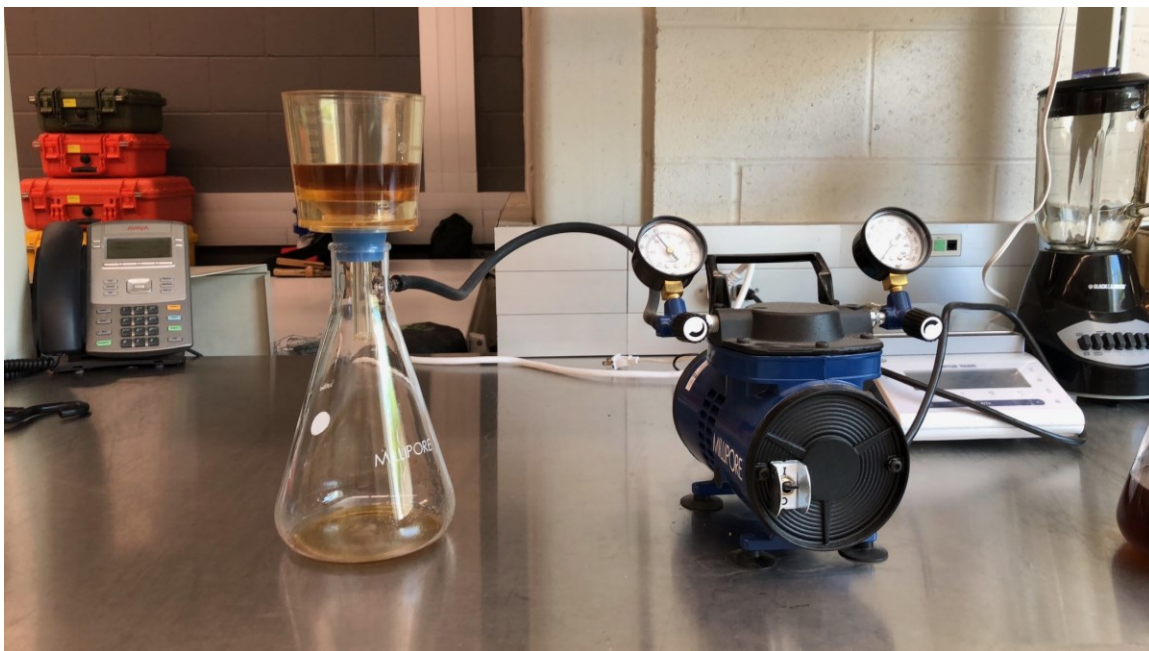
Figure A3. Apparatus used to separate the plant material from the aqueous extract after 24 hours on the shaker. The vacuum pump on the right pulled the aqueous extract through successive filters of decreasing pore size (25 \mu\text{m} , 2.5 \mu\text{m} and 0.45 \mu\text{m} ) into the side arm flask.
