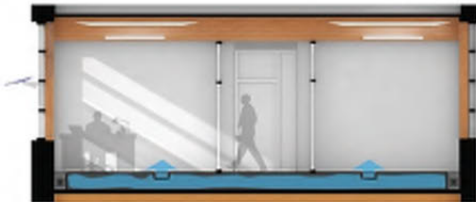
Figure 3: Section/perspective of the diffusers in the raised floor (CIRS Manual).
