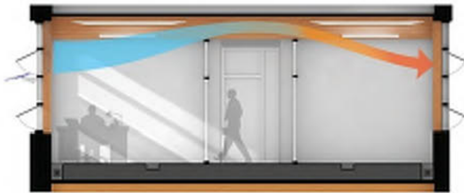
Figure 2: General cross ventilation diagram (section/perspective) in open-plan office areas in CIRS (CIRS Manual).
