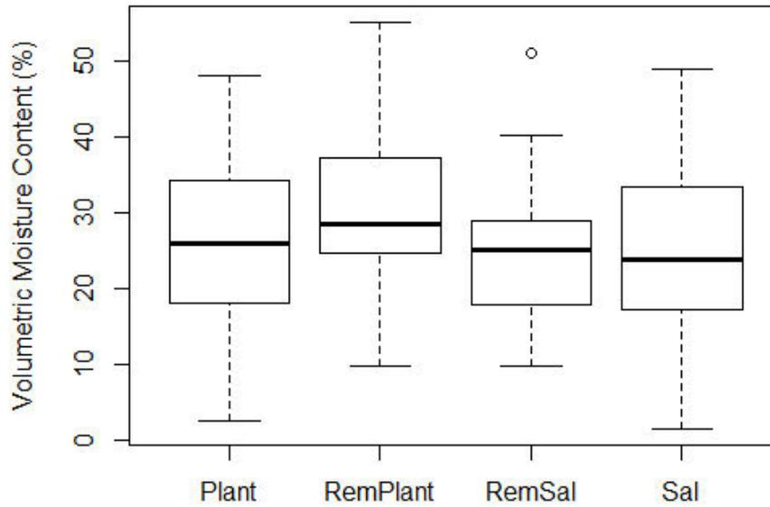
Figure B.7. Soil moisture boxplots. The variation between the treatments is roughly equal and therefore meets the requirement of the one-way ANOVA.
