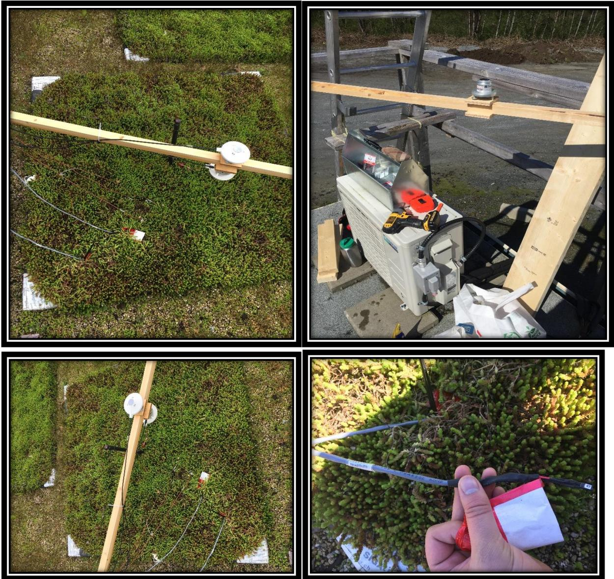
Figure 32. Additional sensors. Top and bottom left – a view of installed sensors; top right – the pyrgometer before installation; bottom right – RH sensor installation.
