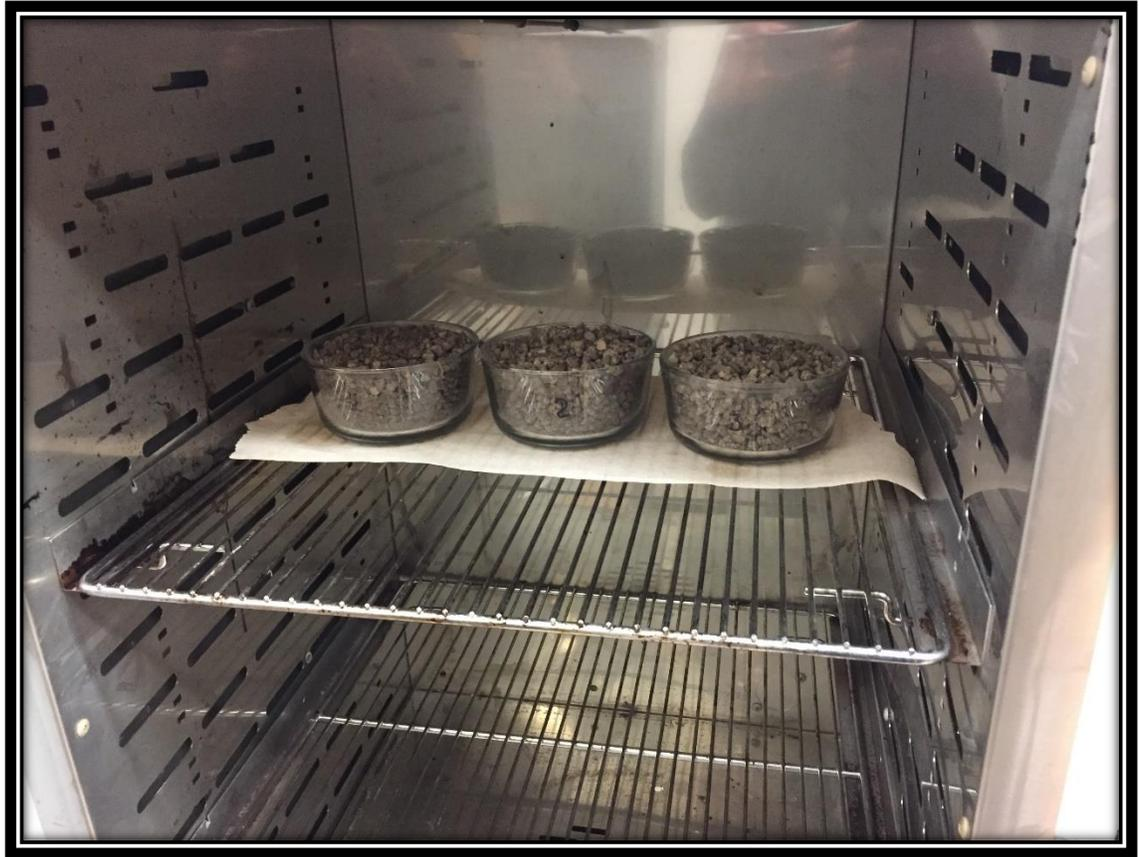
Figure 15. Soil specimens in the oven.
