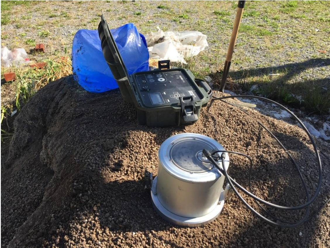
Figure 19. Liquid permeability test.
