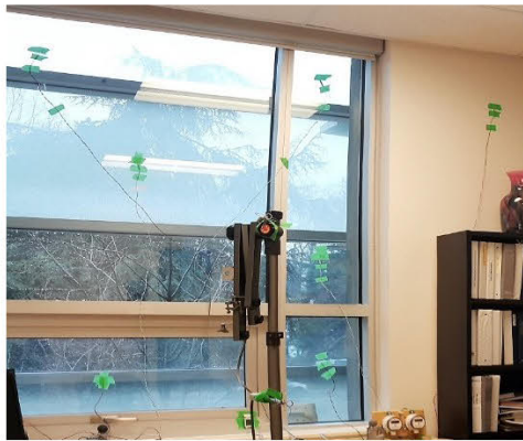
Figure 7.27 - Surface Temperature Measurement - Window and Wall
