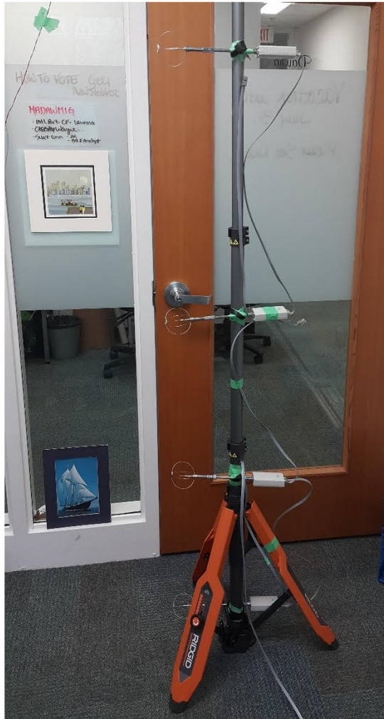
Figure 7.11 - Manifold to Measure Air Velocity and Air Temperature at 4 Different Heights
