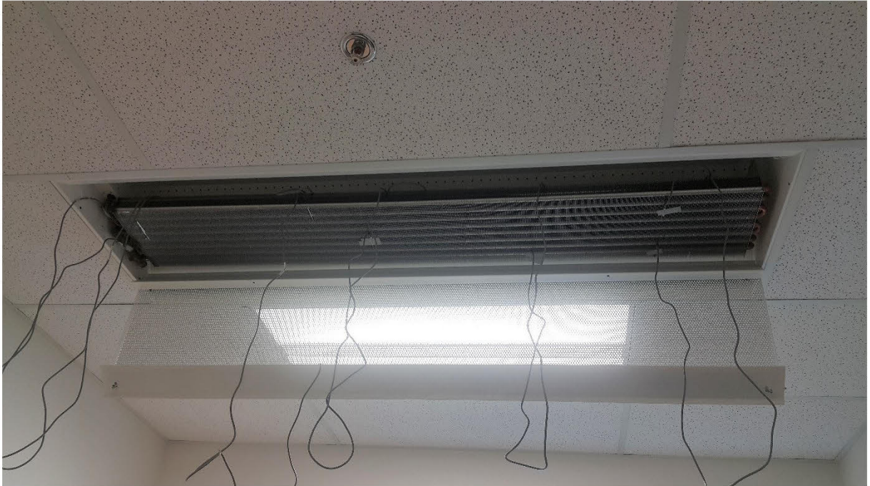
Figure 7.31 - Coil Surface Temperature Measurement
