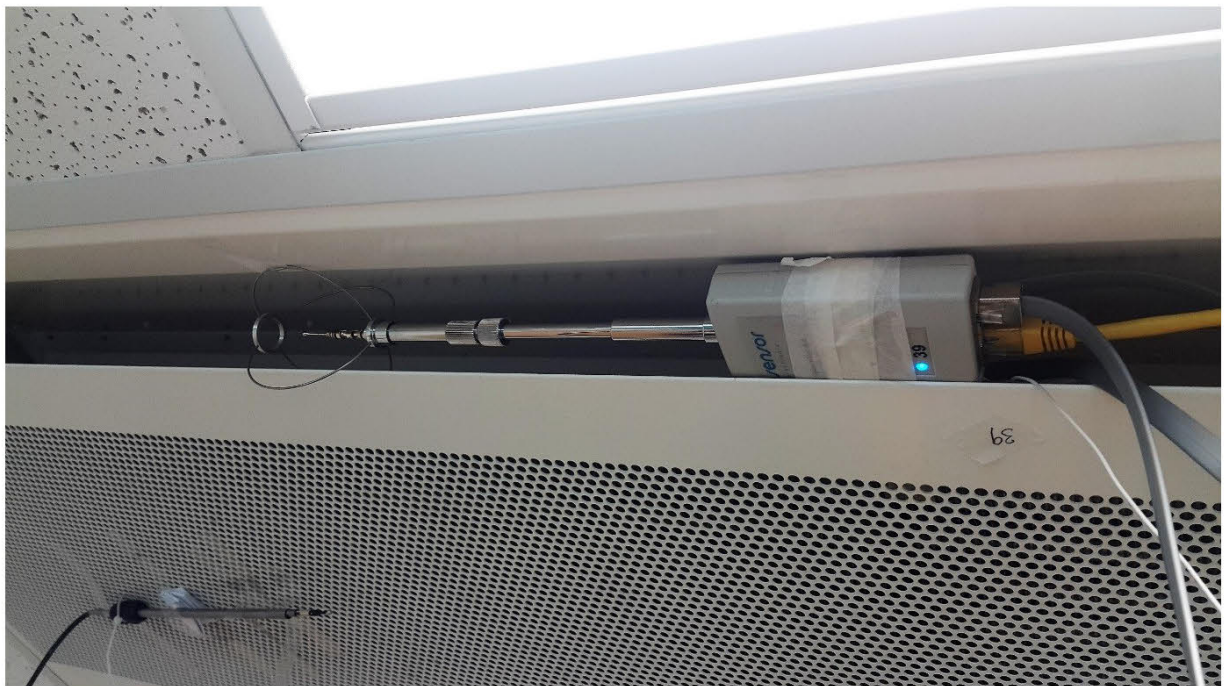
Figure 7.17 - Measurement of Discharge Air Velocity inside Supply Slot
