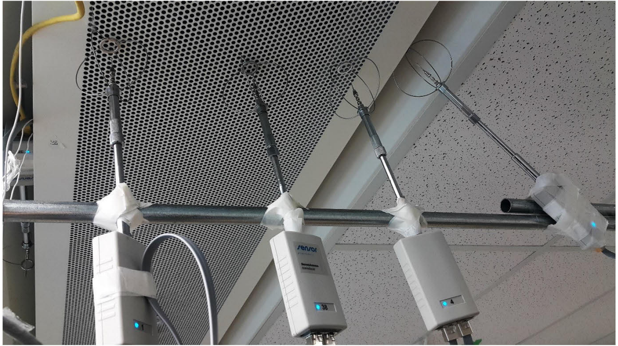
Figure 7.16 – Placement of Anemometers at Induced Surface of ACB
