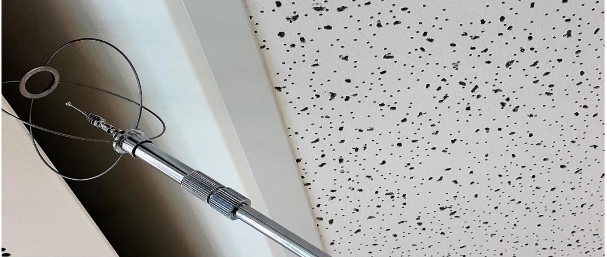
Figure 7.18 - Measurement of Discharge Air Velocity at the Outlet of Supply Slot
