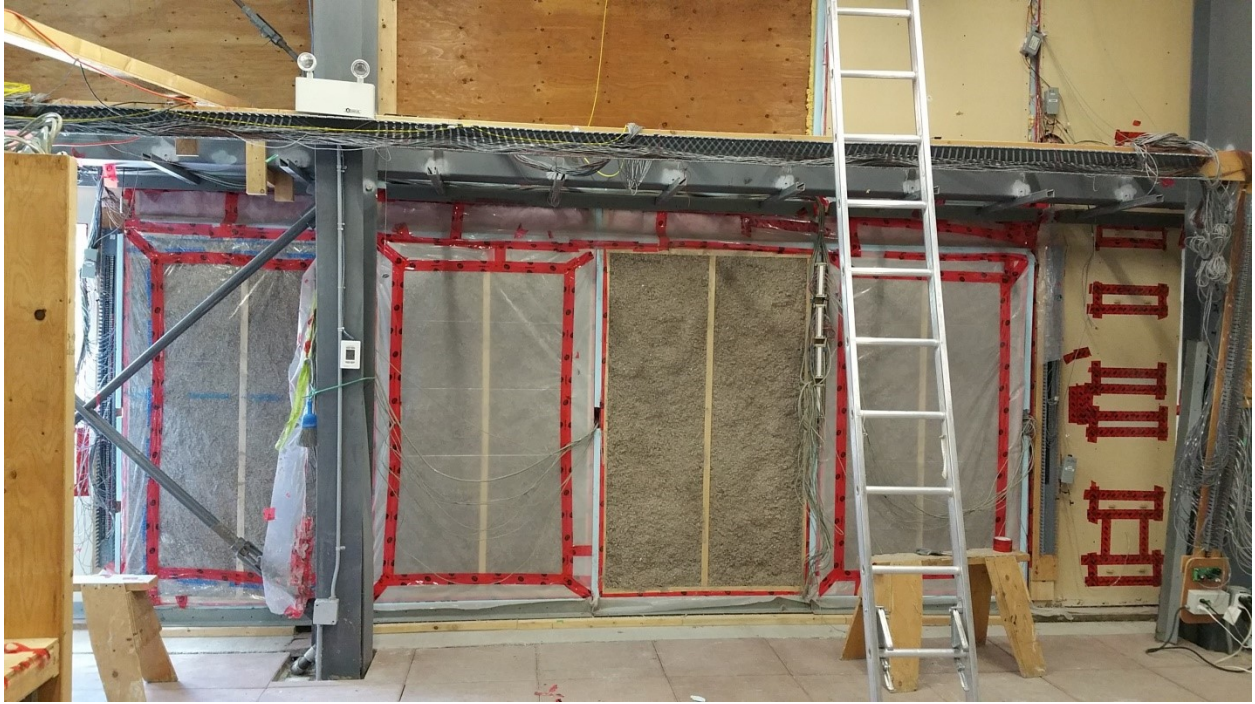
Figure 63- Vapour Barrier Incorporation in Cellulose Test Walls
