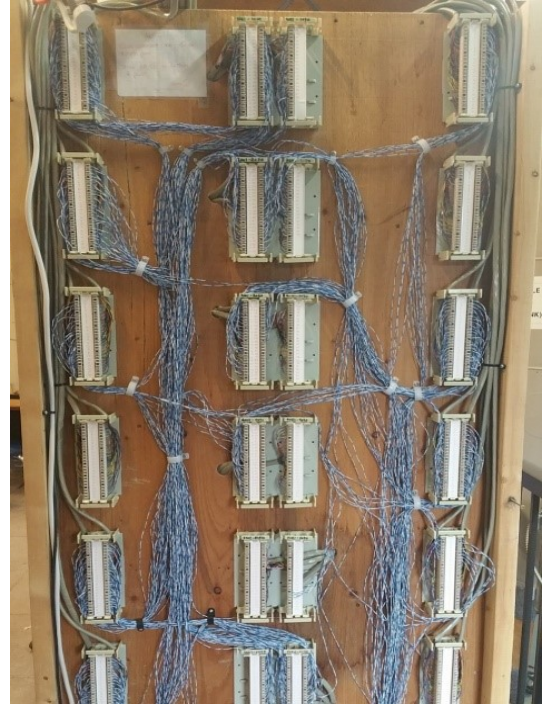
Figure 40- Terminal Strips for Sensors Wiring before DAQ (photo by author)
