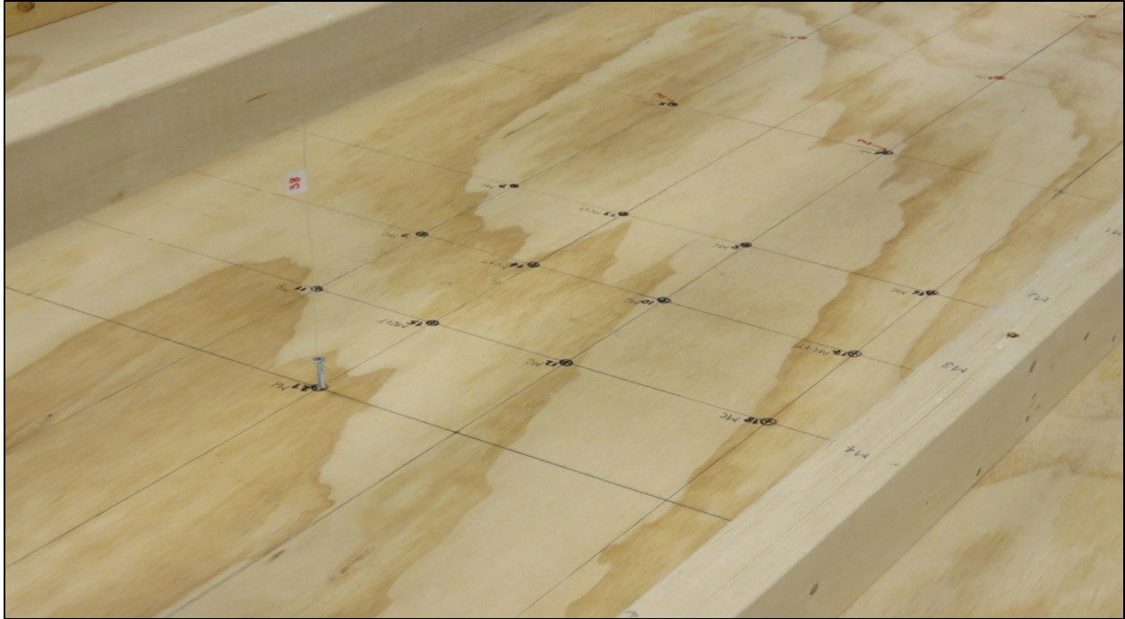
Figure 29- Plywood Sensors Layout (photo by author)
