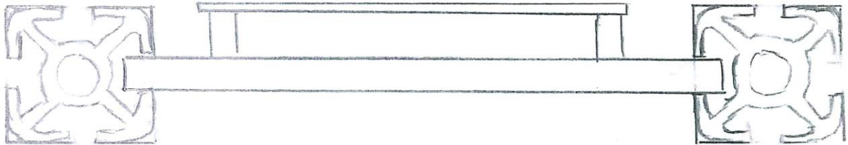
Figure 3.13 - Side extrusion channel supported writing backer
