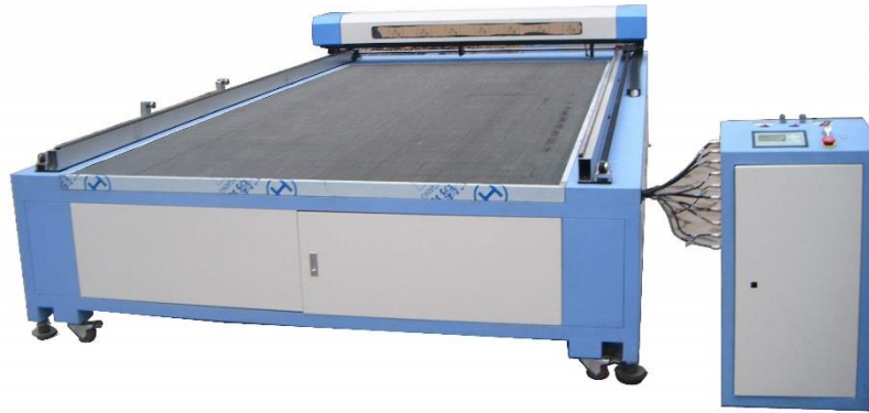
Figure 1.3 - The flat plane that material lies on to be cut by the CNC laser [4]
