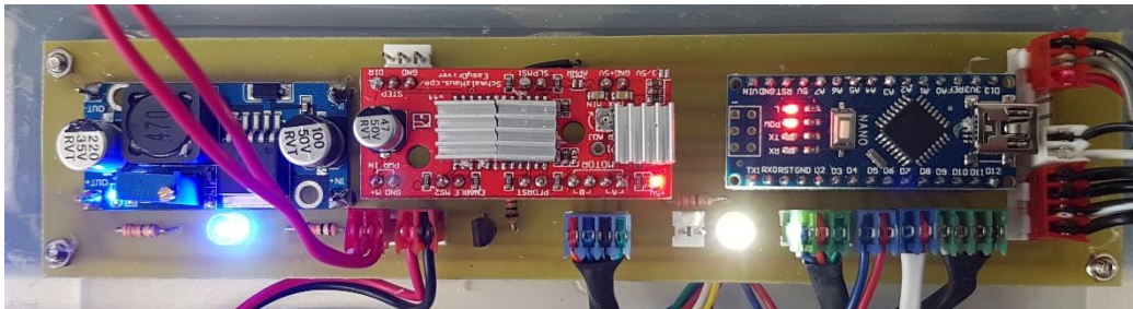
Figure 3.58 - Circuit Board Powered (Limit Switch Activated)
