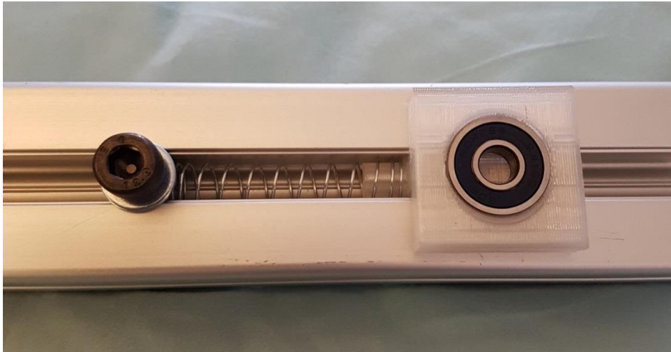
Figure 3.22 - Spring tensioner for rollers
