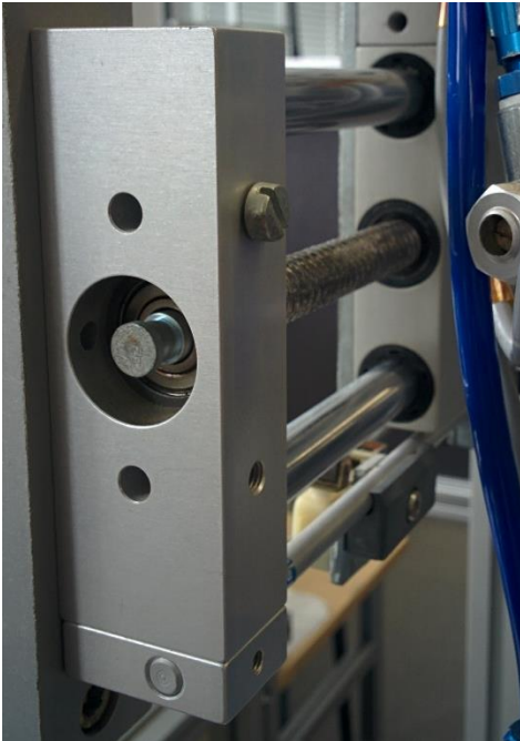
Figure 3.19 - Close up of motion guiding from Festo Didactic
