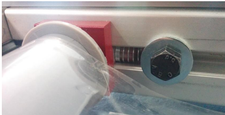
Figure 3.39 - Final spring roller tensioner
