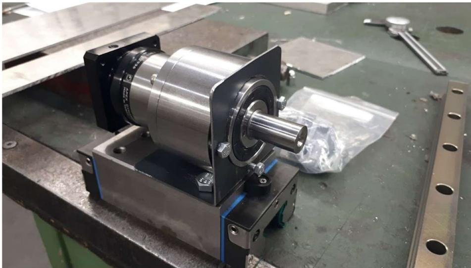
*Figure 4.5 - Gearbox Mounting Bracket*
