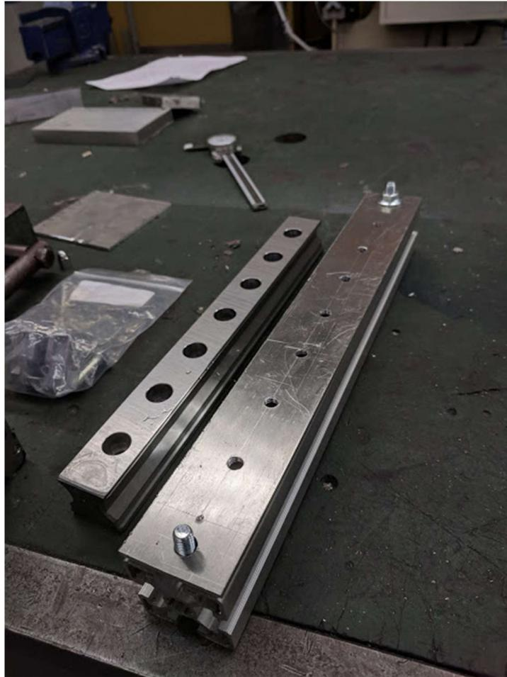
*Figure 4.6 - Linear Slider T-slot Mounting*
