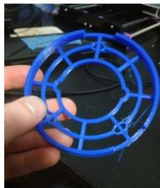
A key feature which is a requirement for passing tech are thruster guards to ensure fingers do not get sucked into the thruster. The company made custom 3D printed guards which attached semi permanently to the thruster. These thruster guards are pictured in Figure 20
