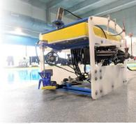
Poly Carbonate part of Electrical housing
