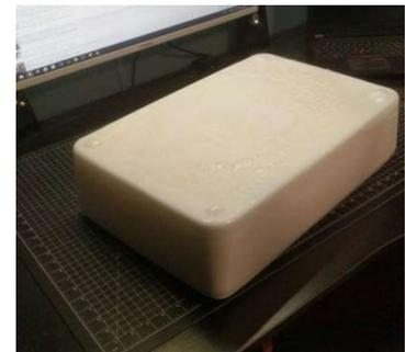
Figure 9 - Foam casting before machining
