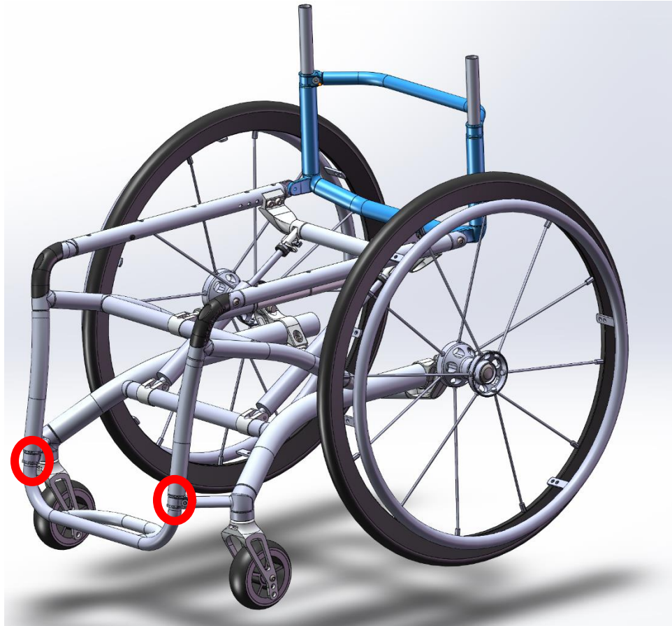
Figure 4 above shows where we plan to apply the strain gauges during the physical validation. We are planning to apply them on both sides of the expected location of highest stress/strain. Which is where the footrest piece is inserted into the frame and clamped. This can be seen closer in Figure 5 below.
