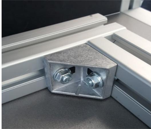
*Figure 4.19 Inside Corer Bracket*
