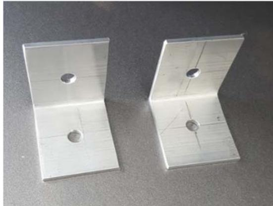
*Figure 4.10 Bearing Block Plate Brackets*
