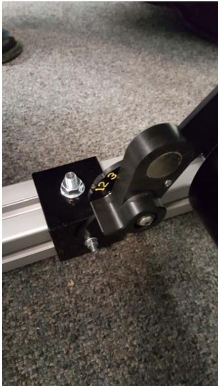
*Figure 5.13 Magnet Resistance Settings*
