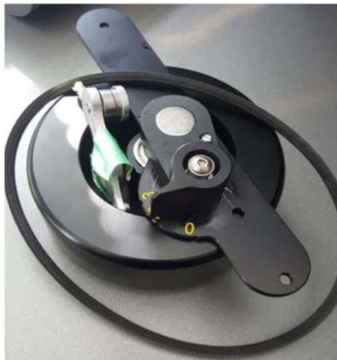
*Figure 4.22 Magnetic Flywheel Assembly*
