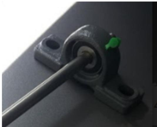
*Figure 4.24 Bearing Block*
