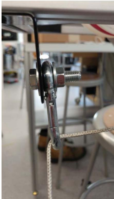
*Figure 5.3 Eye Socket with Nylon Rope*
