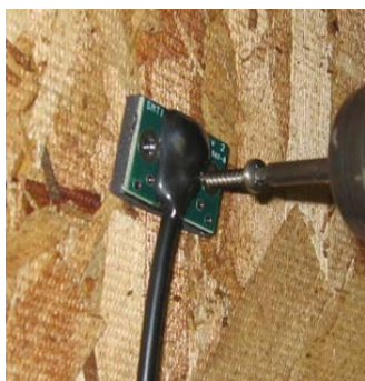
Figure 1. Drive #6 3/4" SS Screw through guides into wood/gypsum.
