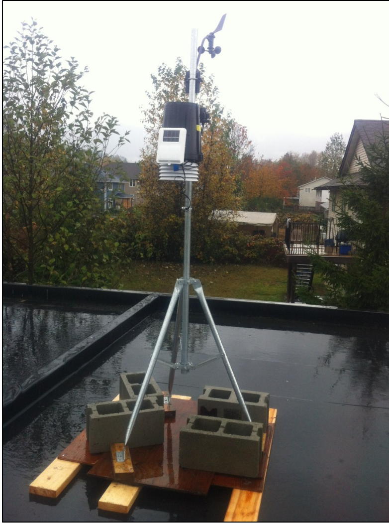
Weather Station Installed on the roof of a building near monitored houses
