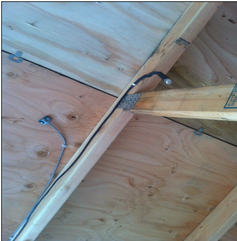
Moisture Content Sensor and Exterior RH/T sensor in the Attic
