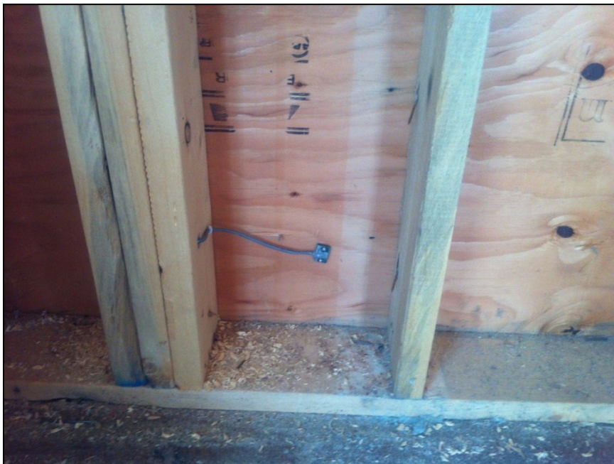
Moisture Content Sensor near the bottom plate below a window
