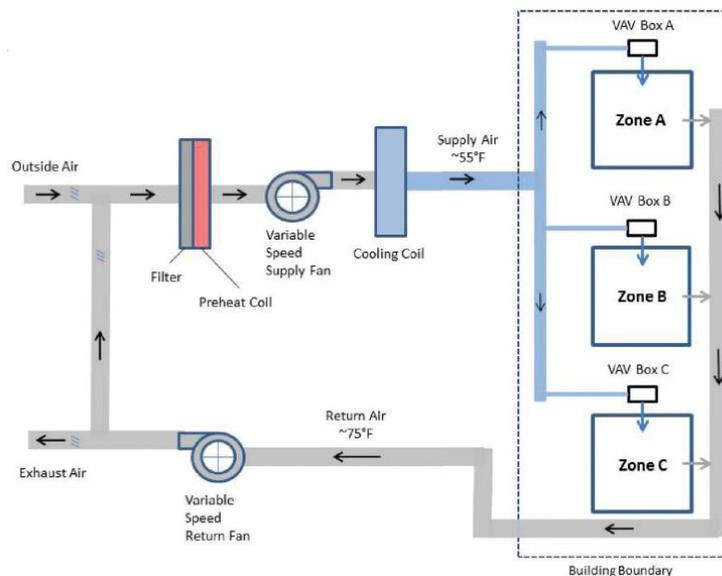
Figure 8. Function of VAV System (Crall, 2015)
