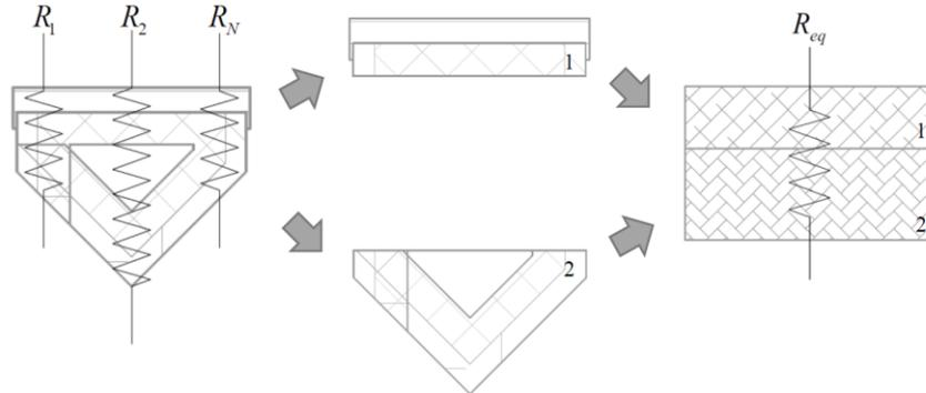
Figure 11. Illustration of Determining U-Value of Specific Masonry Mass Wall
