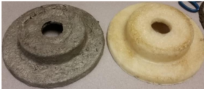
Figure 4-10 - Aluminum Casting (Left) and Polyurethane Mold (Right)
