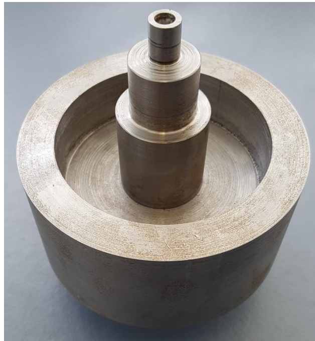
Figure 4-8 - Shaft Mounted in Flywheel
